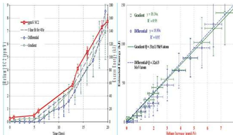
**Figure 3.** Helium production in an LENR experiment at SRI International. *Left:* Time history of the helium concentration in Parts per Million by Volume. *Right:* The excess energy in kJ vs the helium concentration. Fitting the data by different means gave approximately 31–32 MeV per helium atom produced.
