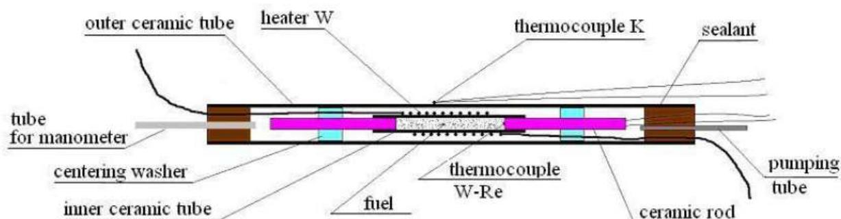
Figure 2. Schematic of the “Protok-6” reactor.
