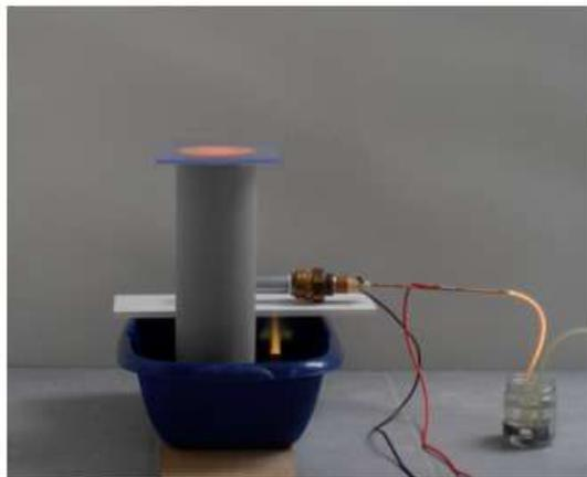
**Figure 21.** Picture taken during a shot. In this case there was no detonation. The protection cover with a foam shock absorber was replaced here by a transparent plastic sheet. The pre-chamber is the steel tube in background. The flame is visible through the cover, as a jet through the gas outlet, and in the transparent gas feeding line up to the gas line isolator on the right of the image.
