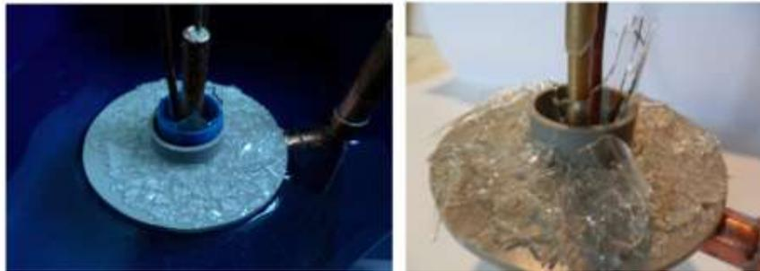
**Figure 22.** Examples of glass debris settled on the tube support after strong detonations. On the left picture, the protection tube has been removed and the water level lowered to make the support visible. On the right picture the assembly has been taken out of the bath. Note that the glass tube section that was immersed in water during the shot is not completely pulverized.
