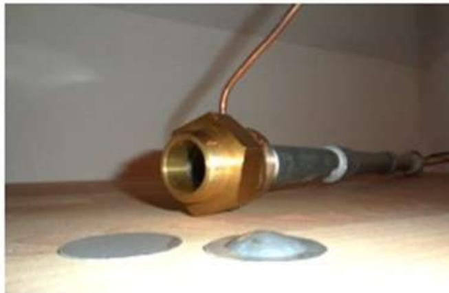
Figure 17. Picture of the reactor steel tube and of aluminum disks before and after a shot.
