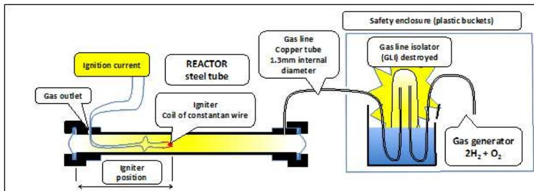
**Figure 19.** Last test of the series in steel tubes. The explosion is transmitted to the GLI and induces an SWACER in the glass tube that is shattered.
