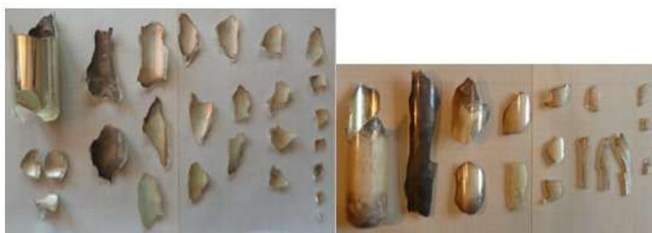
**Figure 5.** *Left:* Pieces from the outer tube. *Right:* Pieces from the inner tube. The cylinders visible on the left of both pictures are parts of the outer and the inner tubes and give the scale.
