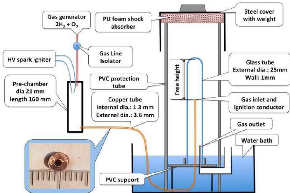
**Figure 20.** The gas is ignited in the pre-chamber. The deflagration propagates along the copper tube to the glass tube. A protection is provided in order to avoid the projection of glass debris by the detonation. The insert shows a cut of the copper tube.
