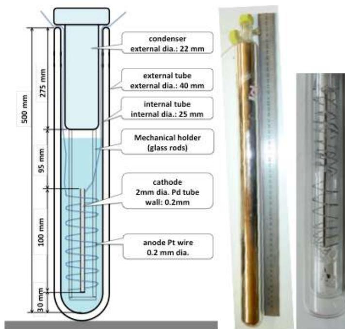
**Figure 2.** *Left:* Schematic geometry of the reactor used during the test with the precise dimensions as shown – *Middle:* The reactor glass tubes were silver coated on the inner faces. *Right:* The electrodes utilized during the test are shown inserted in a similar non-silver coated reactor.
