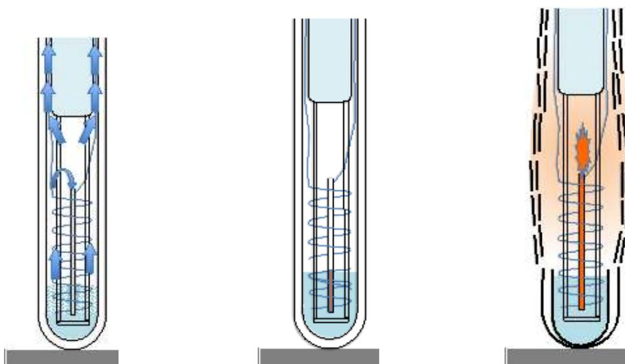
(d) Electrolysis is resumed      (e) Reaction in the hollow cathode      (f) Explosion of the reactor
