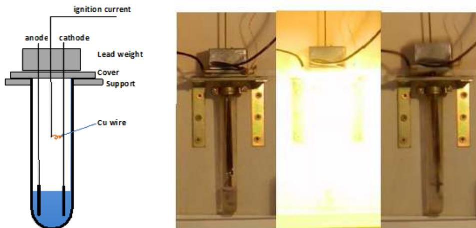
**Figure 15.** Ignition by an exploded wire. The tube is plugged by a lead weight, free to lift under the influence of the gas pressure. Pictures are taken at 33 ms intervals. The maximum altitude reached by the weight makes it possible to obtain a rough estimate of the gas pressure.
