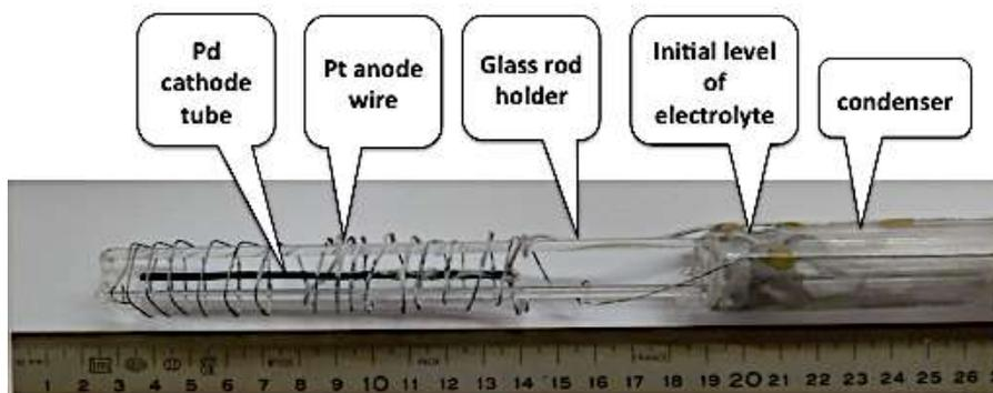
**Figure 4.** Photograph of the electrodes. The ruler shows the altitude over the bottom of the inner reactor tube. Note the trace at 200 mm probably corresponding to the initial level of the electrolyte.
