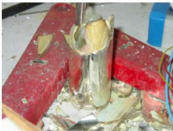
**Figure 3.** Photograph of the reactor after the explosion. The bottom parts remained in place, some liquid was left inside.
