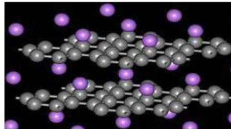
**Figure 2.** Structure of  $\text{CaC}_6$ : violet spheres represent Ca nuclei between layers of carbon nuclei (grey spheres) (after Wikipedia). We may imagine the structure of hydrogen graphite  $\text{HC}_x$  ( $x = 6$  to  $8?$ ) which is not determined yet referring to this structure of  $\text{CaC}_6$ .
