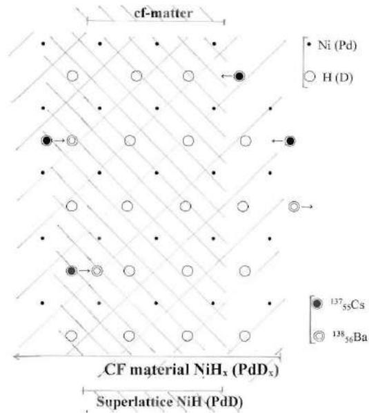
**Figure 7.** Schematic explanation of nuclear transmutations at the surface region of a CF material (e.g.  $\text{NiH}_x$  ( $\text{PdD}_x$ )) in this figure). The nuclear transmutation explained in Section 3.2 (Eqs. (13) and (14)) is illustrated in this figure.
