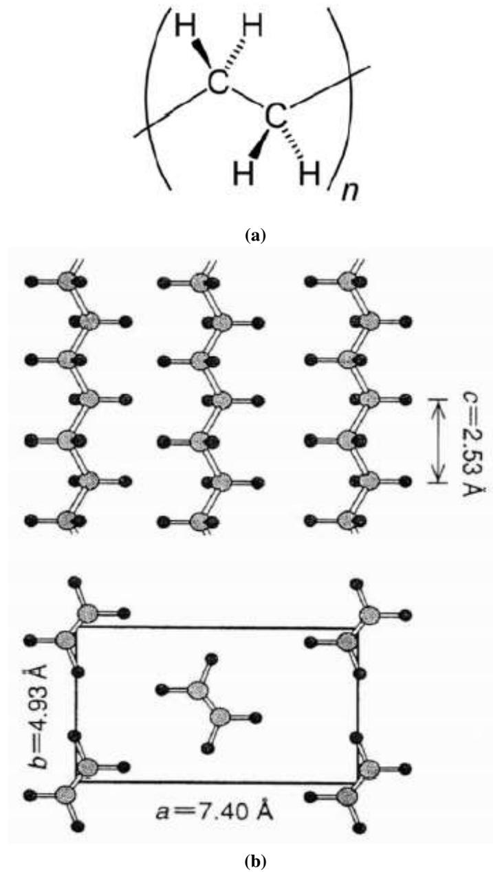
**Figure 3.** (a) Unit of polyethylene  $(C_2H_4)_n$  ( $n = \infty$ ). (b) Lattice structure of XLPE orthorhombic lattice with lattice constants,  $a = 7.40$  (740 pm),  $b = 4.93$  (493 pm) and  $c = 2.53$  (253 pm) ([23], Fig. 5).
