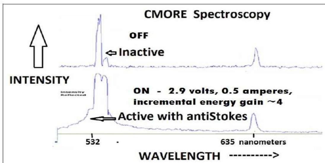
**Figure 3.** Two electric-driven modes revealed by CMORE spectroscopy. This figure shows CMORE spectra. The system used was an aqueous Ni ordinary water system (Pt anode). These are two CMORE spectra of a CF/LANR Aqueous Nickel/H<sub>2</sub>O/Pt system in two electrical states; “off” top, and active XSH mode (*bottom*). Shown are the reflected optical intensities as a function of wavelength (increasing to the right side).
