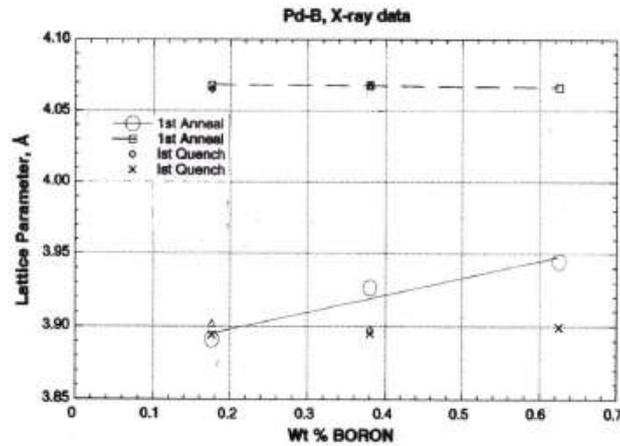
**Figure 5.** Two distinct phases having same crystal structure, but different lattice parameters, are shown. The lattice parameter in a first phase remains constant with changes in the boron content of the alloy, whereas the lattice parameter of a second phase increases with an increase in the boron content.
