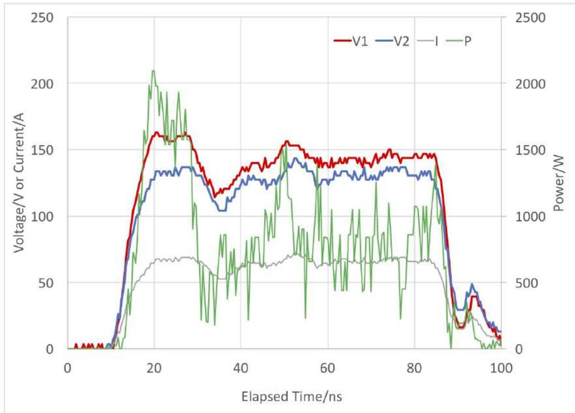
**Figure 4.** Measurement of the Q-pulse power across the tube.
