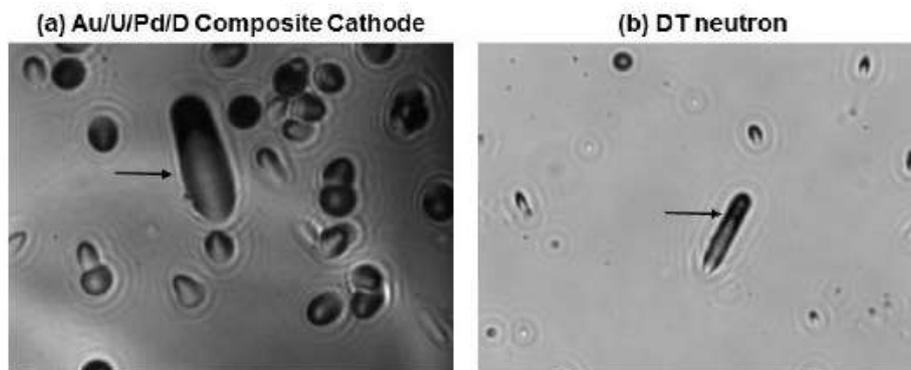
**Figure 4.** Photo micrographs of CR-39 detector that had been used in a Pd/D co-deposition experiment conducted on an Au/U cathode (a) and a detector that had been in contact with uranium wire exposed to DT neutrons (b). Magnification for both is  $1000\times$ . Arrows indicate tracks due to high  $Z$  fragments. The detector used in the co-deposition experiment had been etched for 6 h while the detector exposed to DT neutrons had been etched for 1 h.
