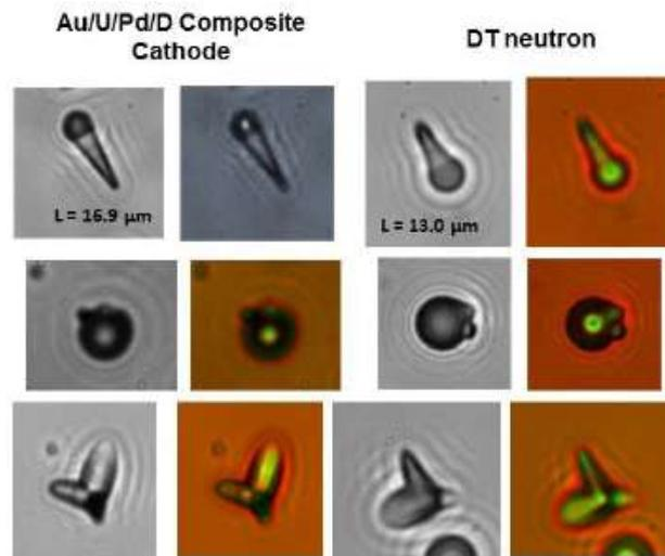
**Figure 3.** Photomicrographs of tracks observed in CR-39 detectors used in Pd/D co-deposition experiment conducted on an Au/U cathode and their corresponding DT neutron generated tracks. Magnification  $1000\times$ . The left-hand images were obtained by focusing the optics on the surface of the detector while the right-hand images are overlays of two images taken at two different focal lengths (*surface and bottom of the pits*). Lengths ( $L$ ) of the recoil proton tracks are indicated.
