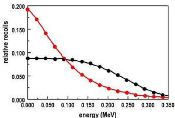
**Figure 2.** Germanium recoil spectra, based on isotropic elastic scattering, calculated for fission neutrons (*red spectrum*) and 6.3–6.83 MeV neutrons (*black spectrum*) using the Monte-Carlo technique.
