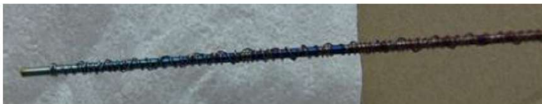
Figure 2. Central discharge electrode. A 250 mm palladium rod, wound with palladium wire.
