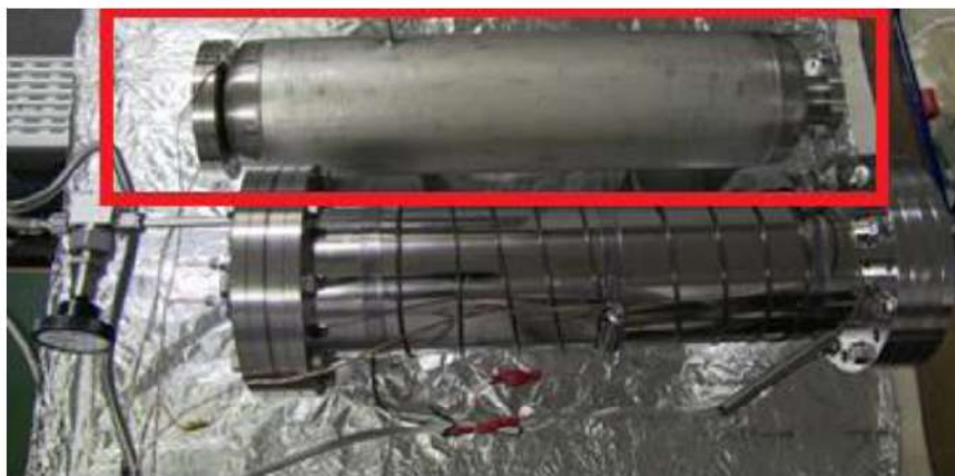
Figure 6. Cylindrical reactors. Length 500 mm, diameter 120 mm, weight 20 kg. A cylindrical reactor and a control reactor ( in red box ) are placed side-by-side in the calorimeter.
