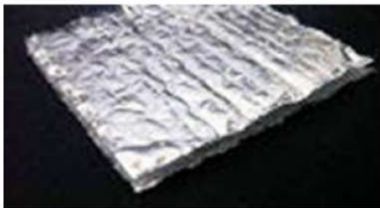
Figure 7. A layer of this reflective padded aluminum insulation is placed on the inside of the box reducing heat leaks to a minimum. At 100–200 W, the inside of the box is only moderately hotter than the surroundings at \sim 36^{\circ}\text{C} , so only \sim 4\% of the heat is lost through the walls and insulation. The rest is recovered in the flowing air.
