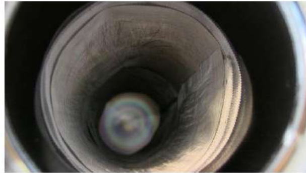
Figure 3. Mesh electrode mounted inside the reactor placed against the reactor wall, connected to ground.
