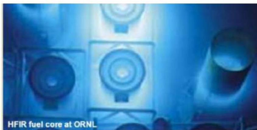
**Figure 2.** Irradiated neptunium at the ORNL fuel core. The blue color is Cherenkov radiation which emanates from spent fuel before it is removed from the High Flux Isotope Reactor (HFIR).
