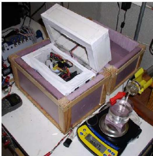
**Figure 6.** Picture of the opened calorimeter with the orphaned oxygen apparatus for measuring the H/Pd atom ratio of the cathode. The calorimeter contains a sealed Pyrex electrolytic cell and a fan. All insides of the box are covered by 54 thermoelectric converters that are maintained at a constant reference temperature of  $15 \pm 0.01^\circ\text{C}$  by flowing water. Measurements are made using NI hardware and LabView. Water enters and leaves the top through the hinges.
