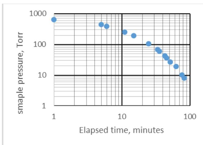
**Figure 1.** Absorption of pure nitrogen in cold traps.
