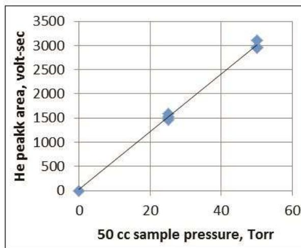
Figure 8. Calibration curve for 12.8 ppm He standard.
