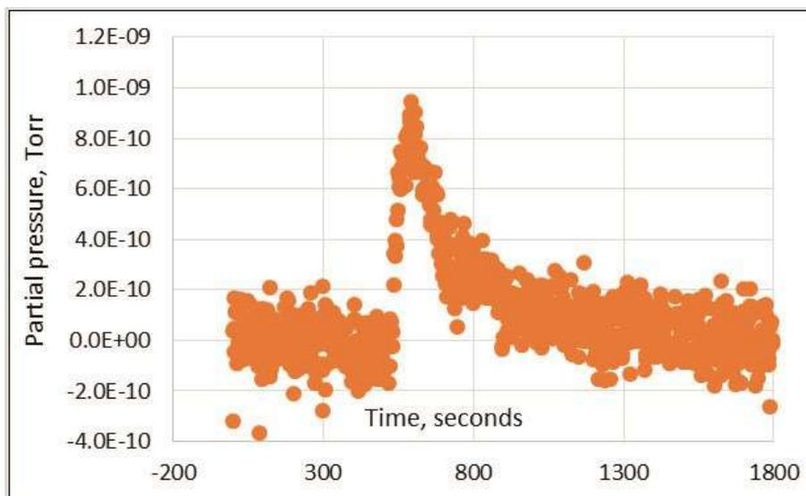
**Figure 5.** Net He-4 RGA signal from 10 cm<sup>3</sup> of air at 2585 Torr.
