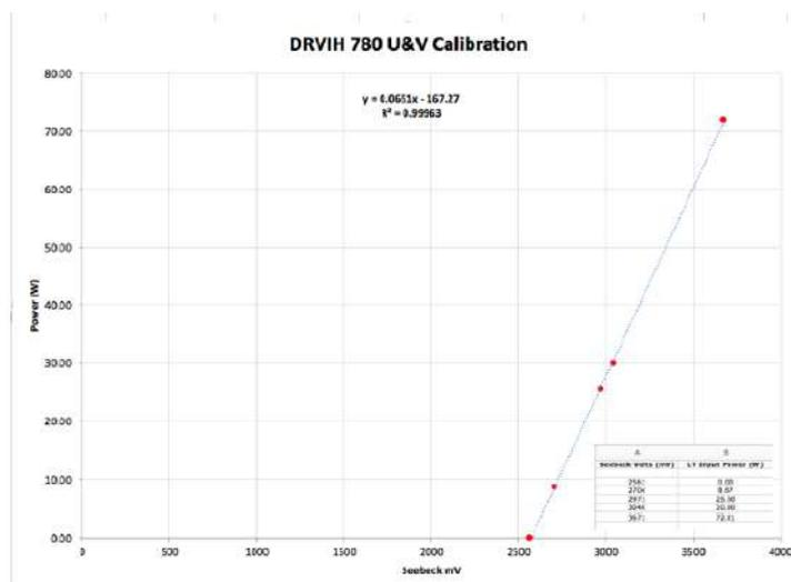
**Figure 9.** A calibration was performed for experiment 780 by adding power to resistive block heaters on top of a steady 200 W that provided baseline operating temperature of about 160°C. The result was a linear calibration plot shown in the figure. The Seebeck reports 2561 mV at zero discharge power because resistance heater power is supplied to provide a minimum operating temperature. Discharge power is applied in addition to baseline heater power.
