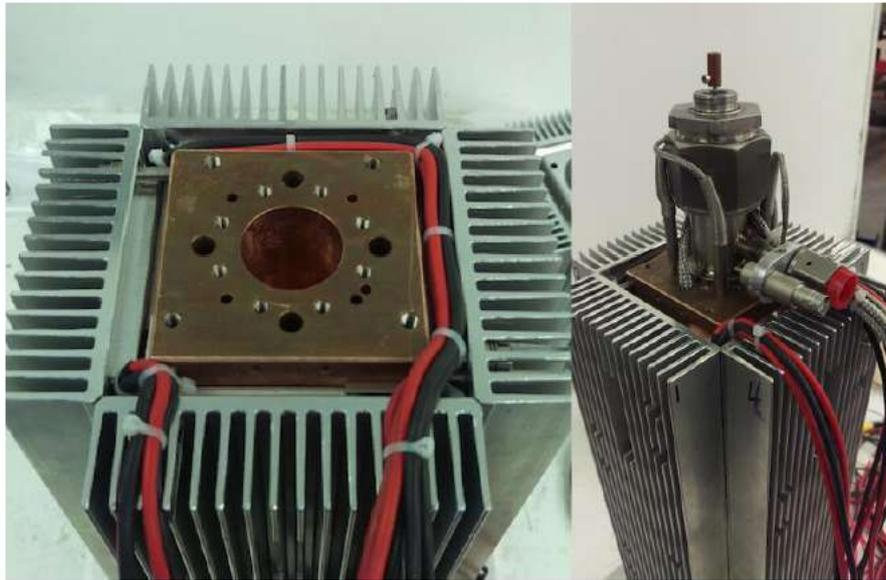
**Figure 3.** The left portion shows the copper block core of the Seebeck calorimeter. The reactor and attached magnets are placed into the central borehole. The larger 1/4 in. holes in the block hold the Watlow resistance heaters that provide minimum heating desired for the reactor. The 1/8th-inch holes are for Omega thermocouples. The right portion shows the reactor in place. A machined lid fits over the reactor and is bolted in place during operation.
