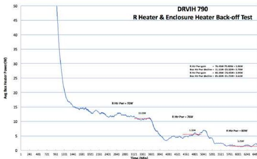
**Figure 14.** The plot shown in the figure shows how the thermal enclosure heater declines in power as a known electrical power is released inside the reactor using the resistance heater shown in Fig. 13.
