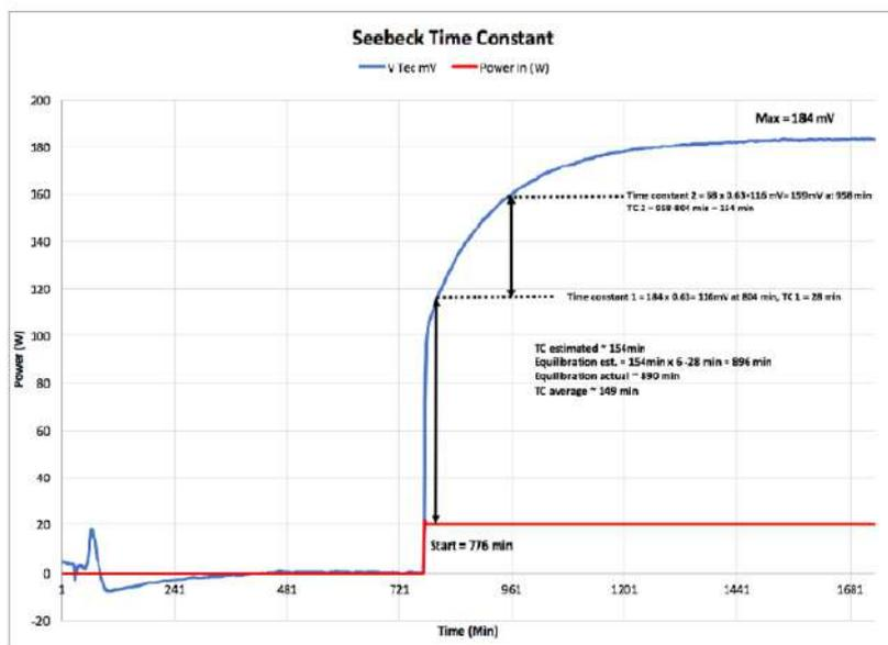
**Figure 8.** The Seebeck has dual time constants, the reason for which is not clear. The TEG manufacturer suggests it may be due to the fact that the thermoelectric devices are a composite of BiTe and PdTe. This plot is NOT for calibration, only to show the time constants of the Seebeck.
