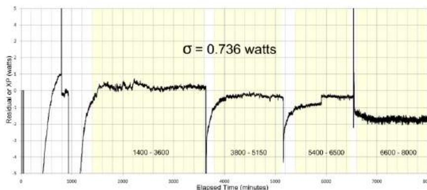
**Figure 15.** Figure shows the standard deviation for power produced in the reactor using the resistance heater shown in Fig. 13. We view the standard deviation as a reasonable measure of calorimeter stability.
