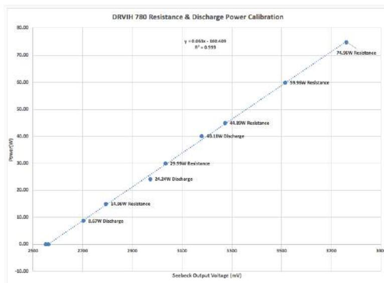
**Figure 11.** Figure shows a calibration made using resistive heating power alone and resistive heating power plus discharge power. The resistive heater only method shown in Fig. 9 produced a higher power output than the method shown in figure by about 1% over the length of the experiment. We chose to use the calibration based on resistive heating power but both calibration methods demonstrated significant excess power and energy.
