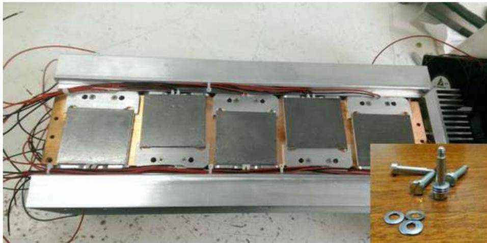
**Figure 4.** Figure shows how the thermoelectric devices are attached to the copper block using Bellville washers, shown in the inset. The Bellville washers provide a constant force to the heat fins as they press against the thermoelectric devices.
