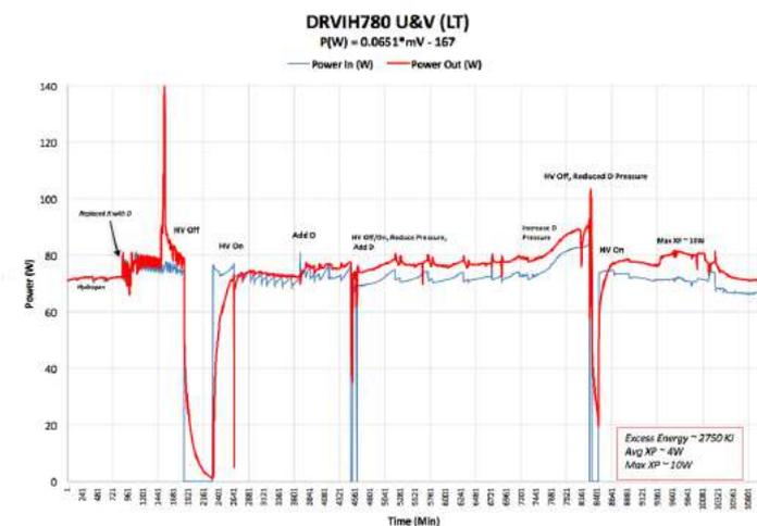
**Figure 10.** Figure shows a long run that produced significant excess power and energy. Of note is the beginning of the experiment where light hydrogen was present in the reactor. After the light hydrogen was replaced with deuterium, excess power appeared and slowly developed over the duration of the experiment that lasted for 7.6 days (11,000 min).
