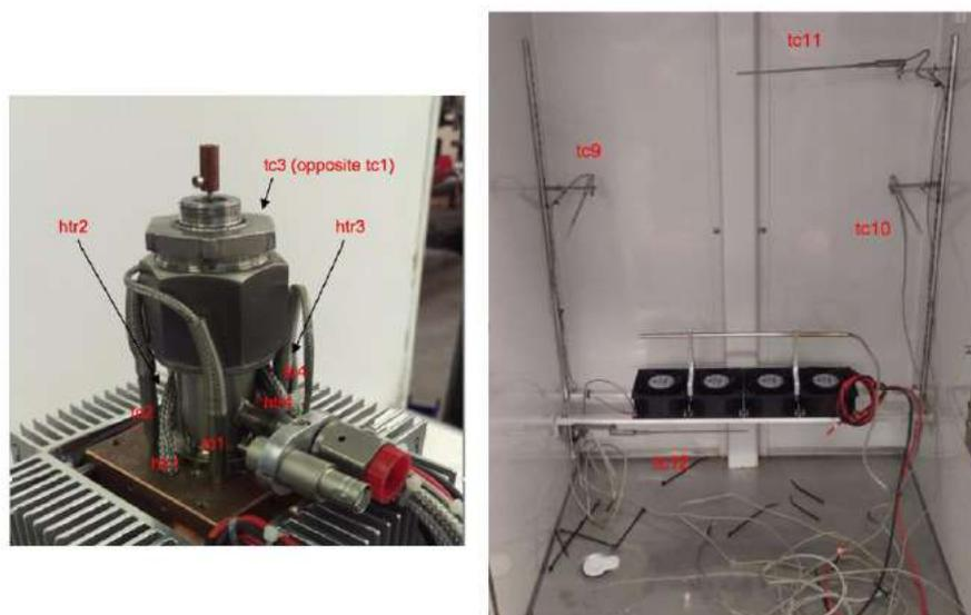
**Figure 5.** Left-hand side shows the positioning of four thermocouples (tc1–tc4) and four Watlow resistance heaters (htr1–htr4). Right-hand side shows the placement of four thermocouples (tc9–tc12) to monitor and control thermal enclosure temperature. Note the Watlow resistance heater above the four stirring fans that is used to keep the thermal enclosure at a constant temperature, as shown in Fig. 6.
