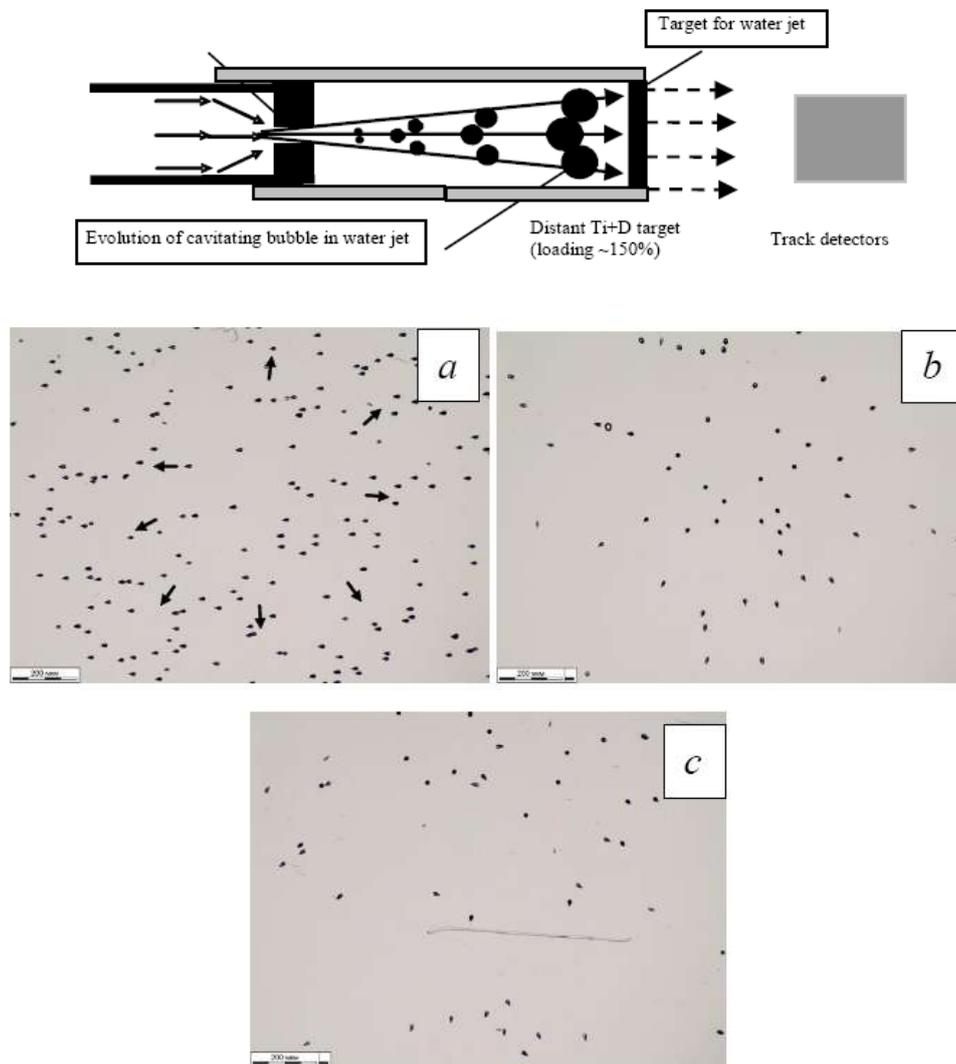
**Figure 2.** Experimental setup and microscopic track analysis of the spatial distribution of tracks and the direction of motion of alpha particles in samples subjected to the action of a thermal wave for 40 min when the track detector is located near the end and lateral (cylindrical) surfaces of the deuterated sample (Fig. 2a,b). (c) Corresponds to a control measurement using an alpha emitter based on a combination of three radionuclides ( $U^{233}$ ,  $Pu^{238}$  and  $Pu^{239}$ ).
