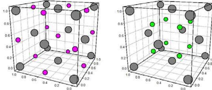
**Figure 7.** Octahedral (*left*) and tetrahedral (*right*) site locations for interstitial hydrogen isotopes in an FCC metal lattice. The locations of the metal atoms are indicated by the larger gray circles. The O-site positions are indicated by the smaller pink circles on the left; and the T-site positions are indicated by the smaller light green circles on the right.
