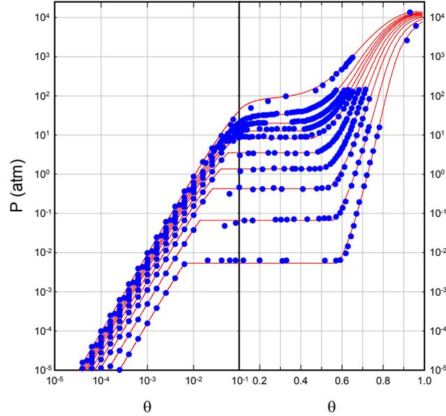
**Figure 4.** Model isotherms (red lines) and input isotherm points (blue circles) for PdH<sub>x</sub>. The isotherms from lowest to highest correspond to temperatures of for (from lowest to highest curves)  $T = 293, 343, 393, 433, 473, 516, 543, 573, 613,$  and  $710$  K.
