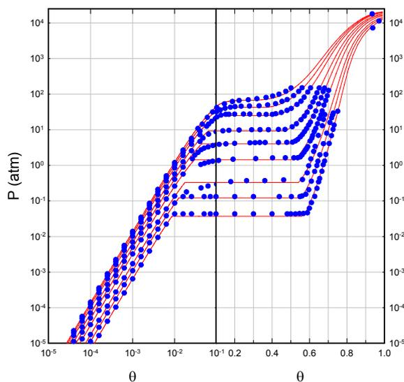
**Figure 2.** Model isotherms (red lines) and input isotherm points (blue circles) for PdD<sub>x</sub>.
