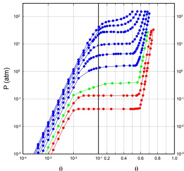
**Figure 1.** Desorption isotherms extrapolated to lower pressure and loading. The circles indicate the loading and pressure data points digitized from [25] in red, [26] in light green, and from [22] in blue; along with extrapolations of the data into the  $\alpha$ -phase.
