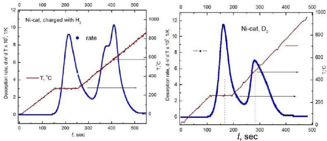
**Figure 5.** TPD spectra of Ni-catalyst charged with  $H_2$  (left panel), to mass concentration 0.13 wt.%; right panel shows TPD spectra for Ni-catalyst sample recharged with  $D_2$ . Mass ratio is 0.24 wt.%.
