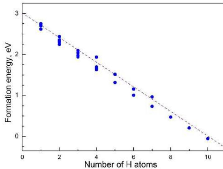
**Figure 2.** Formation energies for various  $m\text{H-V}_2$  clusters with  $m = 0, 1, 2, \dots, 10$ .
