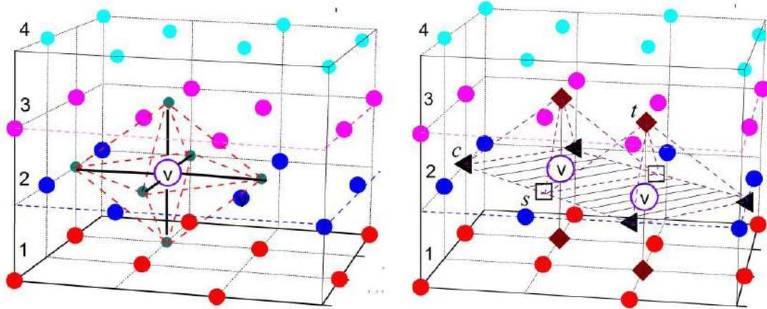
**Figure 1.** Preferred positions of H atoms at octahedral sites in a single vacancy(left panel) and a divacancy formed by emptying two nearest neighbor Ni sites (right panel). Shown is a 32 atom supercell with four atomic layers marked by solid dots of different colors and vacancies shown by hollow dots.
