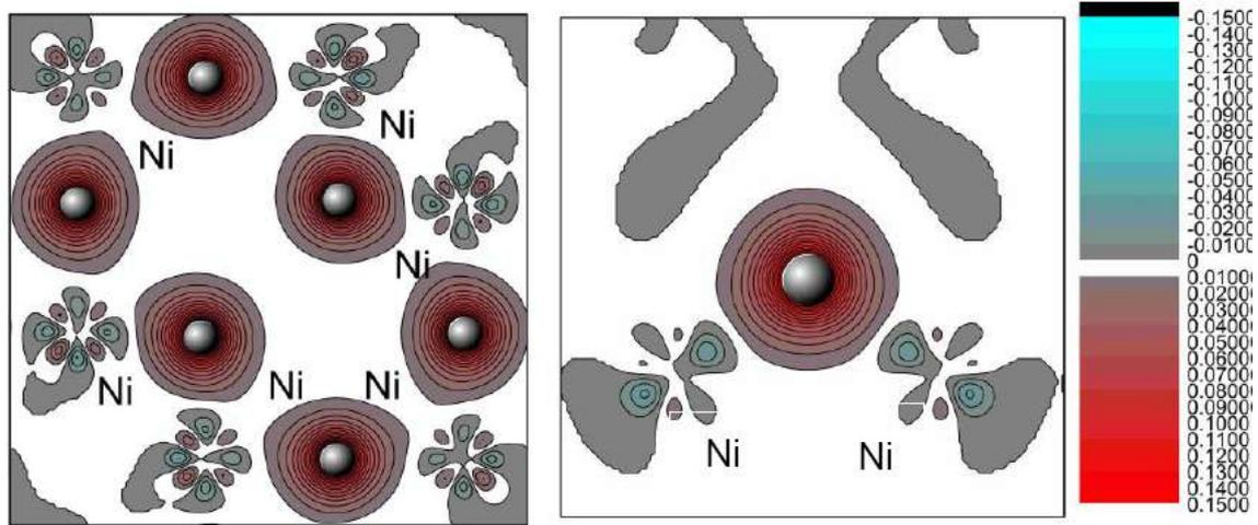
**Figure 3.** Redistribuition of electron density in 10H–V<sub>2</sub> cluster in the divacancy (100) plane (*left panel*) as compared to that for a H interstitial atom at a tetragonal site (*right panel*). Blue and gray contours show depletion regions, pink and red indicate accumulation of electronic clouds around gray balls of H atoms in Ni lattice.
