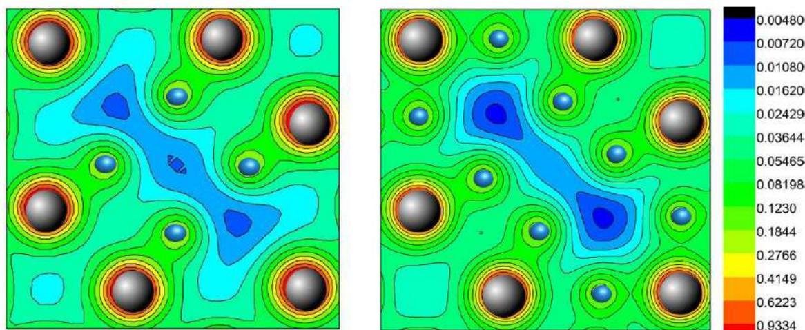
**Figure 4.** Electron charge distribution in (001) plane of  $mH-V_2$  cluster in Ni with 4 and 8 segregated H atoms in anomalous (*pair*) positions with reduced distance between H atoms. Color panel shows density values in atomic units ( $1/au = 6.748 e/\text{\AA}^3$ ). Preferable positions are at the density  $\cong 0.22 e/\text{\AA}^3$ .
