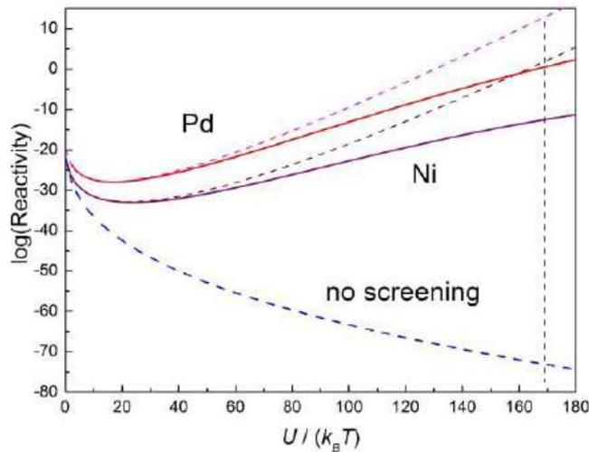
**Figure 6.** Reactivity for D–D reactions in Pd and Ni (in  $\text{cm}^3/\text{s}$  units, log scale) enhanced by the screening factor  $\exp(\Gamma)$ , see Eq. (2), as a function of ratio  $U/k_B T$ ; also shown is the reactivity without screening and reactivities in the local screening approximation (dashed lines).
