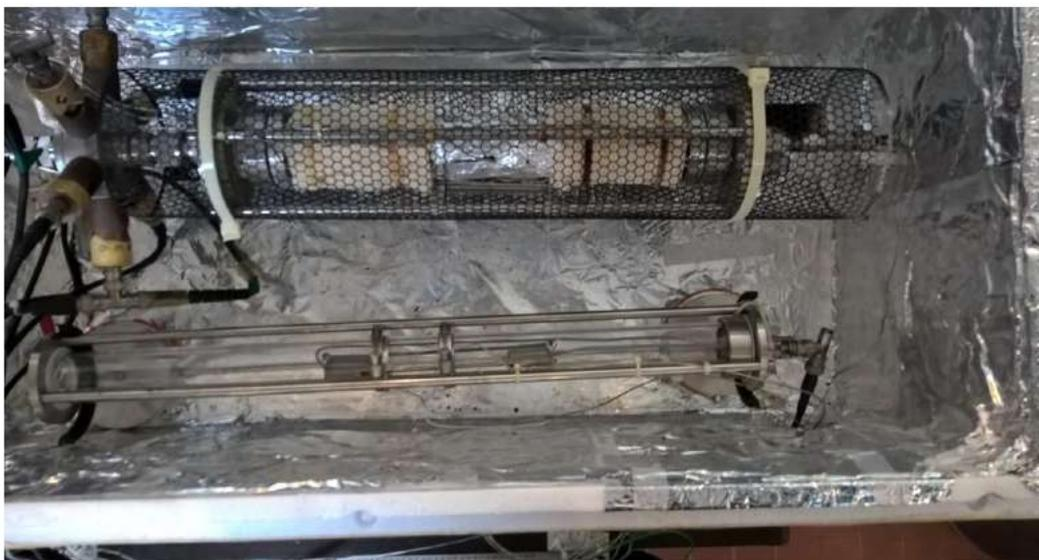
**Figure 10.** Interior of the air-flux calorimeter with the reactor (*above*) and the Halogen Tungsten lamp used for calibration (*below*, max power 230 W). The lamp is inserted inside a borosilicate glass tube of the same dimensions of that used for the reactor. The internal walls of the insulating box are covered with an aluminum foil in order to make temperature as uniform as possible inside the calorimeter.
