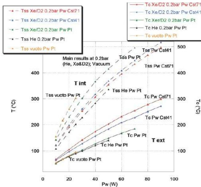
Figure 3. Temperature versus Input Power applied to the reactor in vacuum ( $P_w$  at Pt), He ( $P_w$  at Pt), Xe+D<sub>2</sub> mixture ( $P_w$  at Pt, Cst41, Cst71) atmosphere. A large increase of external temperature  $T_c$  is observed with respect to Pt case for  $P_w$  applied to Cst41 and Cst71.
