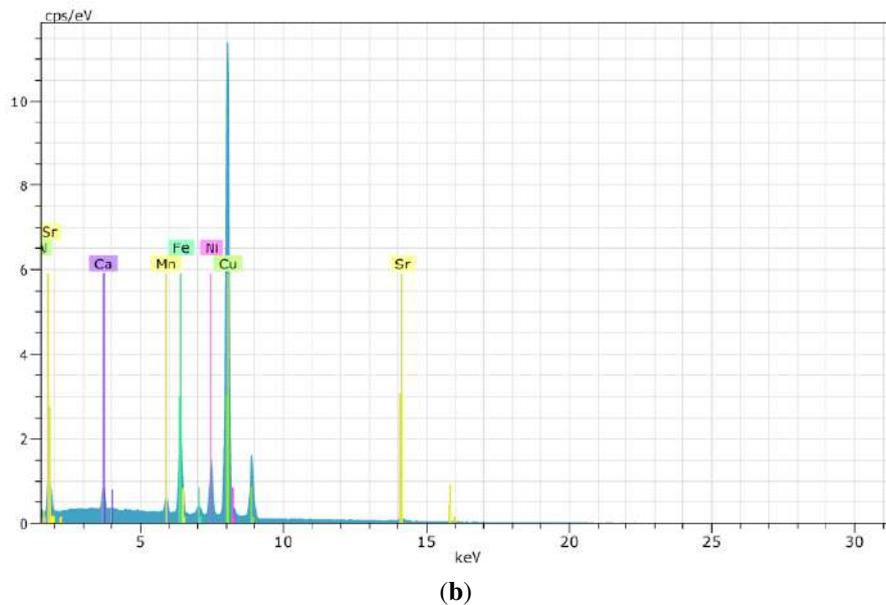
**Figure 6.** (a) SEM observation of a typical area at the top of the knots (wire with  $\Phi = 200 \mu\text{m}$ ). (b) Corresponding EDX spectrum. Surface element composition changes remarkably after the application of HPP procedure, particularly as regards Nickel.
