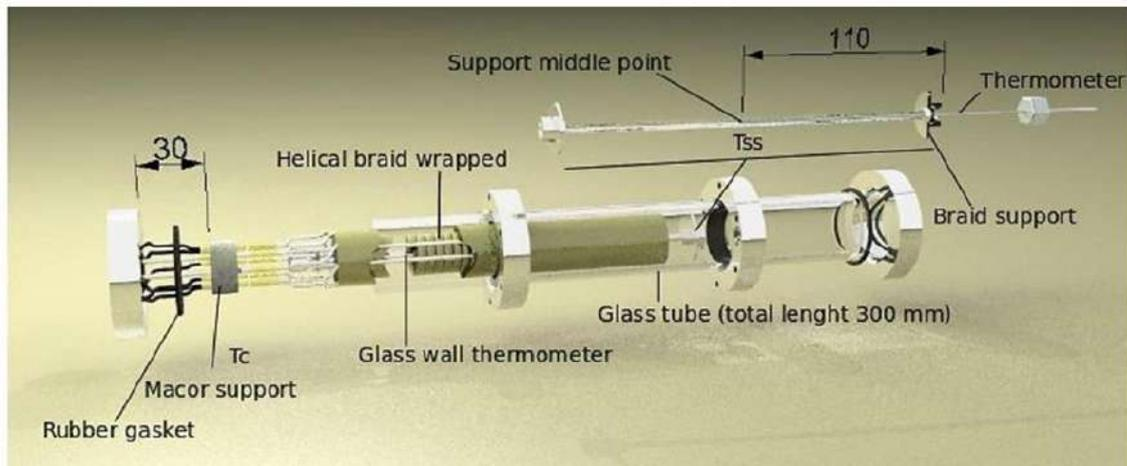
Figure 2. Schematic of the reactor once assembled.
