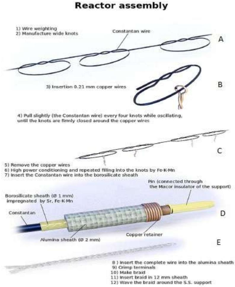
**Figure 1.** Reactor assembly: (A) Preparation of the knots in the constantan wire. (B) Insertion of the copper wires in order not to completely tighten the knot. (C) Critical point of tightening the node due to possible stress of the constantan wire. (D) After conditioning, insertion of the wires inside the several glass sheaths. (E) Braid of the three wires to be waved around the SS support.
