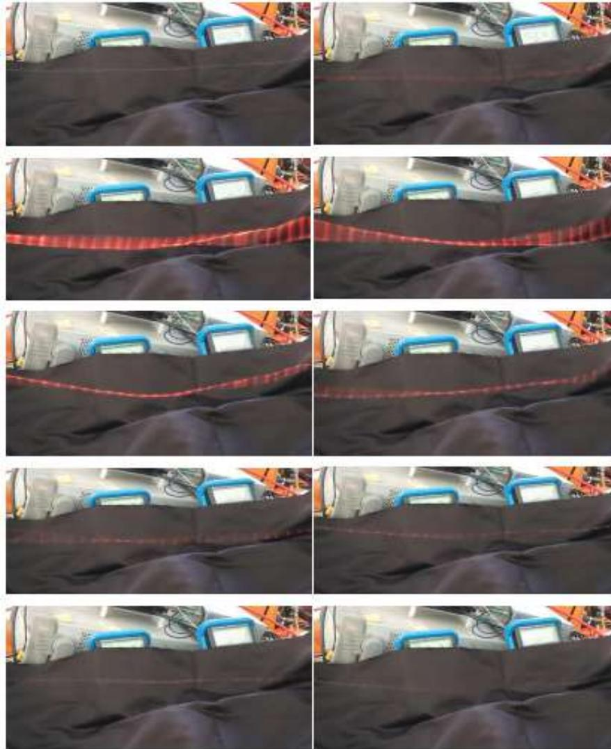
**Figure 4.** Photographic sequence of a 200- $\mu\text{m}$ -diameter constantan wire subjected to High Peak Power Pulses: the time frame is about 20 ms and pulse duration is 70 ms. The brighter dots along the wire correspond to the knot sites, which reach higher temperatures than the other parts of the wire. In this way, local thermal non-equilibrium conditions are achieved.
