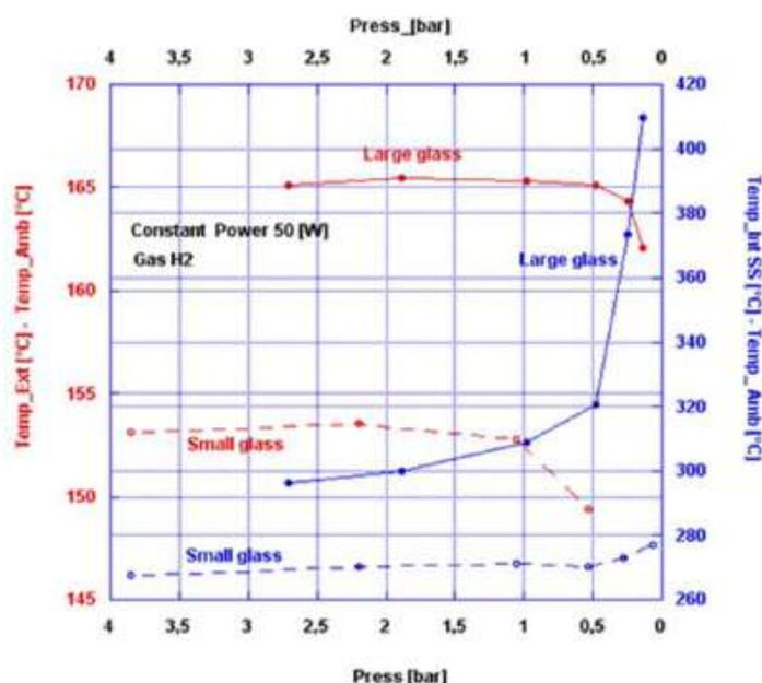
**Figure 9.** Data comparison for tests conducted with a small and a large amount of glass enveloping the SS support in the reactor, in  $H_2$  atmosphere and at constant input power of 50 W. Temperature difference with ambient at the external glass tube surface (red) and at the central SS tube (blue) is plotted against pressure in the reactor.
