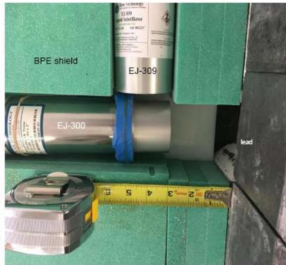
**Figure 17.** Shielded scintillators.
