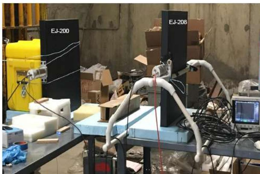
**Figure 16.** AmBe neutron TOF calibration in Igloo.
