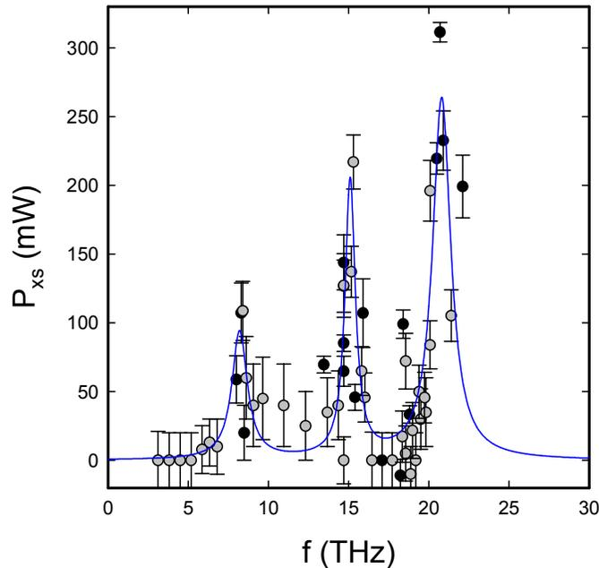
**Figure 4.** Excess power (mW) as a function of difference frequency (THz). Data from step results as in Fig. 3 are in black; data from scans are in grey. Best fit of three Lorentzians shown as a solid line.
