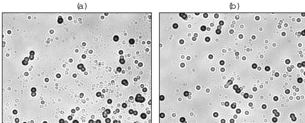
**Figure 12.** Photomicrographs obtained at 500 $\times$  magnification for (a) Pd/D codeposition tracks and (b)  $\sim$ 1 MeV alpha tracks. (a) and (b) reprinted with permission from *J. Condensed Matter Nucl. Sci.* [35].
