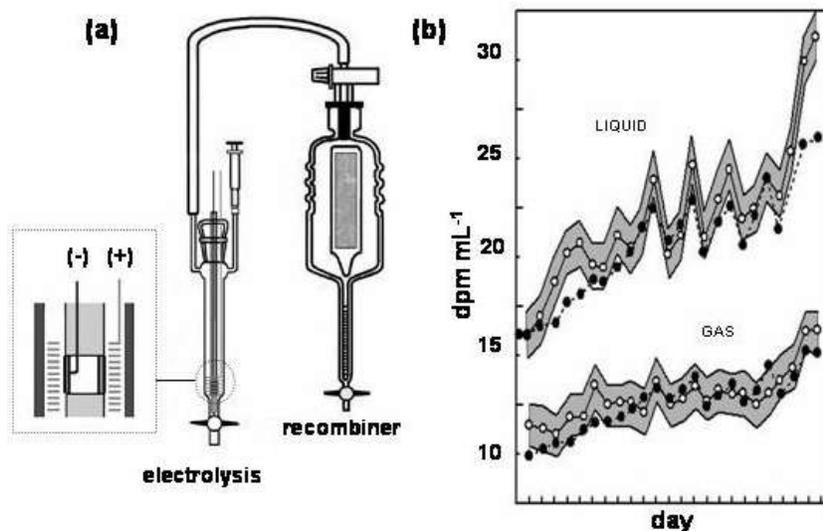
**Figure 3.** (a) Schematic of the electrolysis cell and recombiner used to monitor tritium in the gas and liquid phases during electrolysis. (b) Tritium content, in  $\text{dpm mL}^{-1}$ , for Pd/D co-deposition done on a Cu/Ag/Pd cathode. Open circles are the experimental data with the  $2\sigma$  error bars, solid circles are the amount of tritium expected based upon the mass balance.
