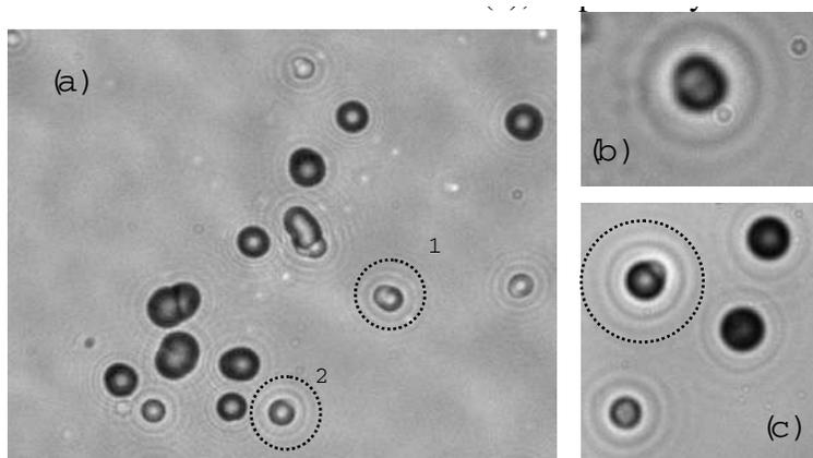
**Figure 9.** (a) Pd/D co-deposition tracks at 500 $\times$  magnification. (b) and (c)  $\sim 1$  MeV alpha tracks obtained by placing 24  $\mu\text{m}$  of Mylar between a CR-39 detector and an  $^{241}\text{Am}$  source. Images (b) and (c) taken with a magnification of 1000 $\times$ . [23] (Reprinted with permission from *Eur. Phys. J. Appl. Phys.*)
