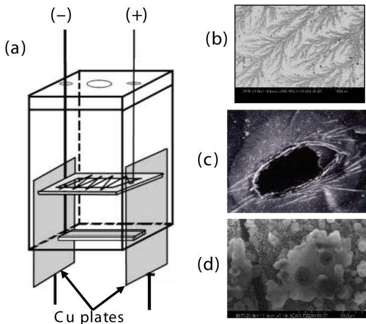
**Figure 5.** (a) Schematic of the cell used in the external electric field experiment. SEM images of the Pd deposit upon termination of the experiment showing (b) fractals, (c) craters [15] (Reprinted with permission from *J. Electroanal. Chem.*), and (d) micro-volcano like features.
