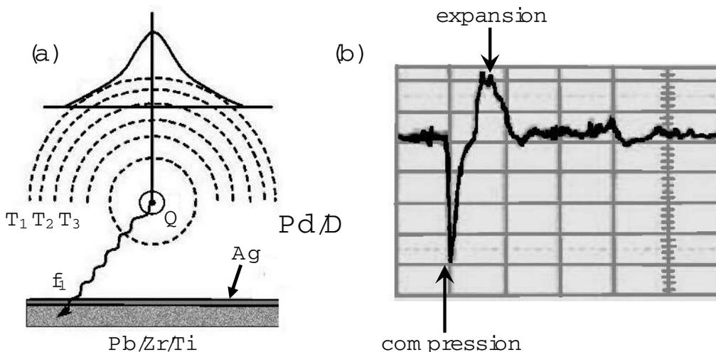
**Figure 4.** (a) Schematic of the events that should occur when a mini-explosion occurs during Pd/D co-deposition. (b) A recording of a single mini-explosion that was detected using a Pb/Zr/Ti piezoelectric crystal.
