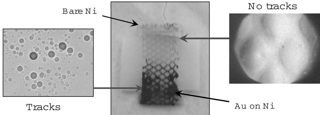
**Figure 10.** Results obtained on a CR-39 detector used in a Pd/D co-deposition experiment done in the absence of an external field. A photograph of the cathode is shown in the middle. Photomicrographs of the CR-39 are shown.
