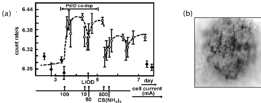
**Figure 2.** (a) Count rate during cathodic polarization of the Cu/Ag/Pd electrode as measured using a HPGe detector. The period of Pd/D co-deposition is indicated as well as the addition of LiOD and CS(NH<sub>2</sub>)<sub>2</sub>. (b) Fogging of photographic film after exposure to Pd deposited on an Ag disk cathode [6] (Reprinted with permission from *Eur. Phys. J. Appl. Phys.*). A thin Mylar sheet separated the film from the cathode.
