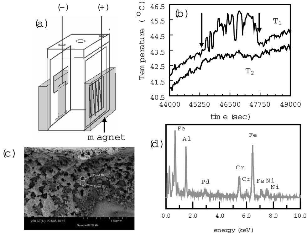
**Figure 6.** (a) Schematic of the cell used in the current external magnetic field experiment. (b) Temperature response of the Au/Pd cathode ( $T_1$ ) and solution ( $T_2$ ) for an experiment conducted in the presence of a 120 G magnetic field. Cell current was at  $-400$  mA. Arrows indicate when the electromagnet was turned on and off. (c) SEM of Pd deposit exposed to a 2500 G external magnetic field. (d) Elemental analysis of point 10 in (c).
