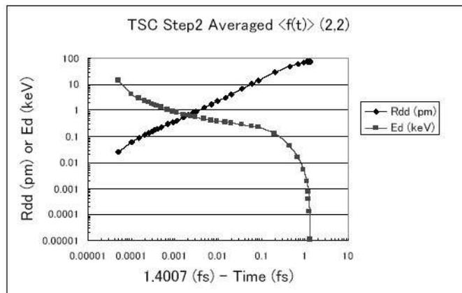
**Figure 9.** Numerical solution of Eq.(13) by the Verlet method<sup>4</sup>. Time is reversed starting from the condensation time at 1.4007 fs.
