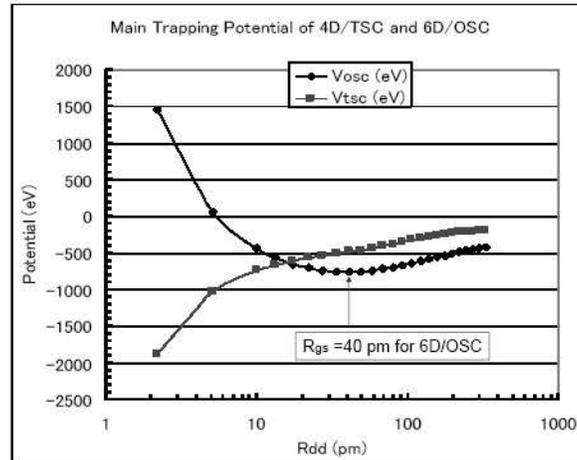
**Figure 8.** Comparison of cluster trapping potentials for 4D/TSC and 6D<sup>2-</sup>/OSC. TSC condenses ultimately to a very small  $R_{dd}$  value ( $R_{dd} - min = 20 fm$ ), while OSC converges at  $R_{dd} = 40 pm$  (corresponding to the ground state).
