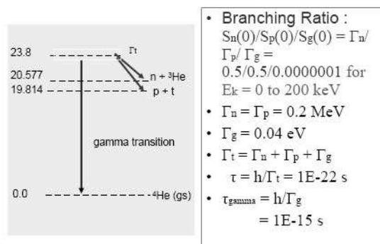
Figure 2. Break-up (out-going, decay) channels of  $d + d$  fusion.
