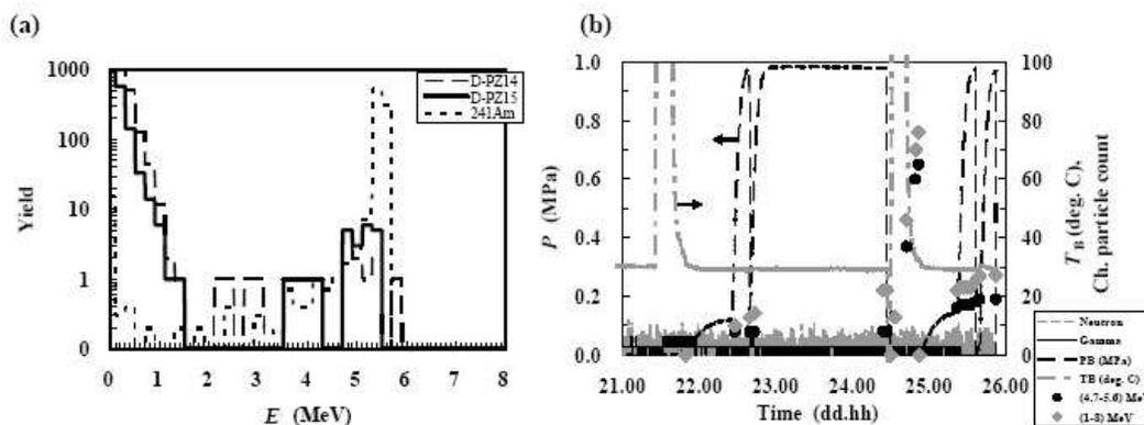
**Figure 7.** (a) Spectra recorded by the IISD with a 500- $\mu\text{m}$ -thick depletion layer and (b) Evolution of pressure and IISD counting and other radiations during the runs D-PZ14#1B through D-PZ15#2B.
