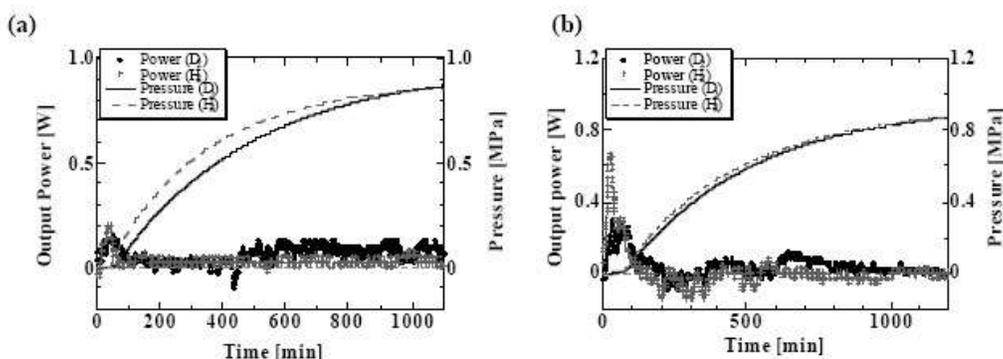
**Figure 3.** Evolution of heat and pressure in the vessel after pumping D<sub>2</sub> gas or H<sub>2</sub> gas; (a) 0.1- $\mu\text{m}\phi$  Pd powder (D-PP1#1 and H-PP2#1), (b) 300-mesh Pd-black (D-PB1#1 and H-PB2#1).
