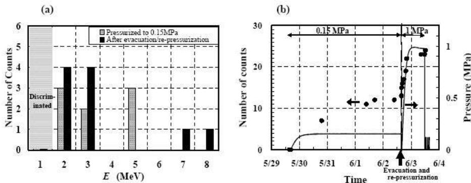
Figure 6. (a) Spectra recorded by SSBD with a 200- $\mu\text{m}$ -thick depletion layer and (b) Evolution of counting in the “1–12 MeV” range of the spectra measured by the SSBD during the run DPZ1# 3B through D-PZ1#4B.
