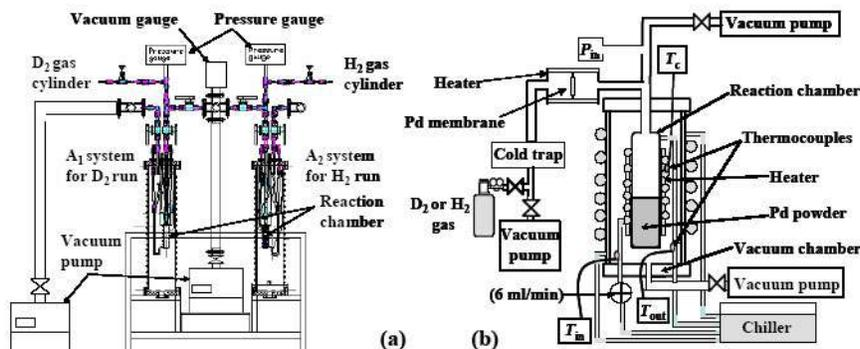
**Figure 1.** (a) Reduced view of the A<sub>1</sub> · A<sub>2</sub> twin system, and (b) functional view of A<sub>1</sub> used in the early stage of the present research. The Pd membrane filter for flow rate control is replaced by a mechanical needle valve, ‘Super Needle’.
