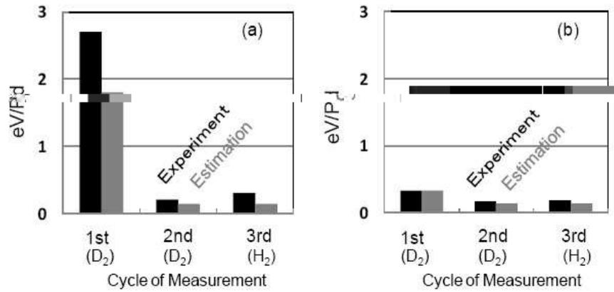
**Figure 9.** Variation of heat generated in the first stage with cycle of measurement for (a) 20 wt.%Pd- $\gamma$ Al<sub>2</sub>O<sub>3</sub> and (b) Pd nanopowder AY4030. Experimental values are compared to the estimated ones.
