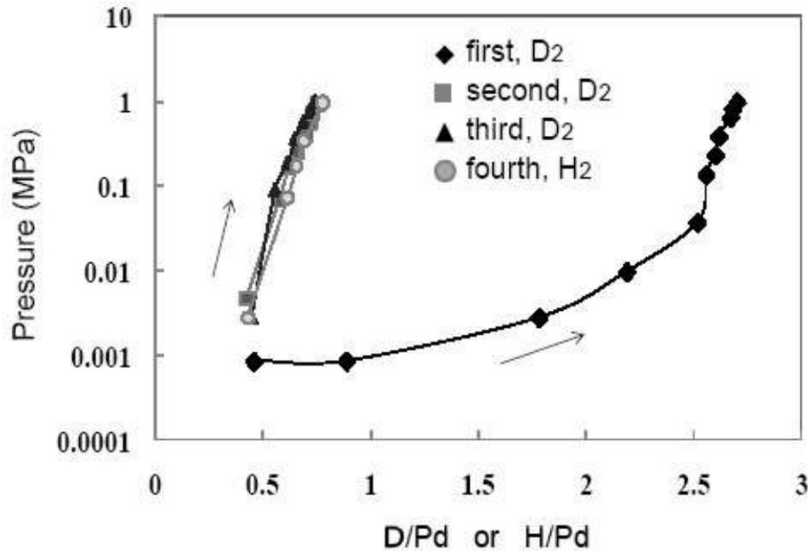
**Figure 5.** PC isotherms of 13 wt.%Pd- $\gamma$ Al<sub>2</sub>O<sub>3</sub>. Isotherms were measured four times repeatedly. The arrows show the sequence of the measurements.
