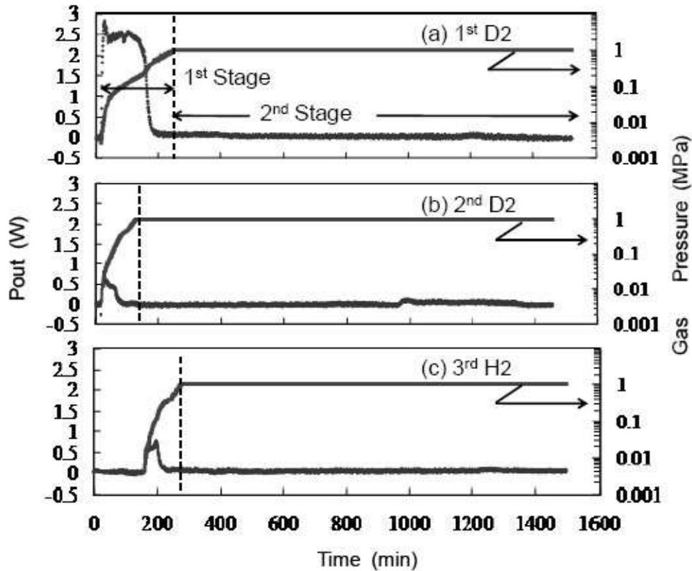
**Figure 8.** Heat power and gas pressure as a function of time for 20 wt.%Pd- $\gamma$ Al<sub>2</sub>O<sub>3</sub>; (a) the first cycle loading with D<sub>2</sub>, (b) the second cycle loading with D<sub>2</sub>, (c) the third cycle loading with hydrogen.
