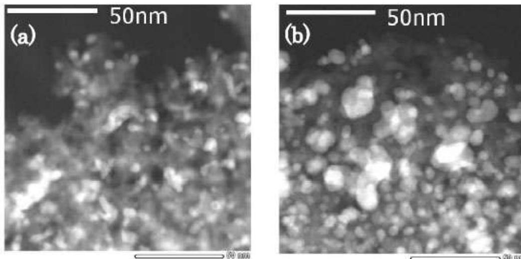
**Figure 7.** Scanning TEM images of 13 wt.%Pd- $\gamma$ Al<sub>2</sub>O<sub>3</sub>; (a) as-synthesized, (b) after four cycle measurements of absorption capacity. The white spots are PdO (a) or Pd (b).
