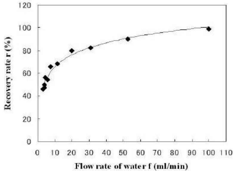
**Figure 2.** Recovery rate ( $r$ ) as a function of flow rate ( $f$ ) for Pd nanopowder AY4030 of 26 g under a He gas pressure of 0.85 MPa. The electric input power was 1.5 W or 0.66 W. The solid line is drawn to connect the data points smoothly.
