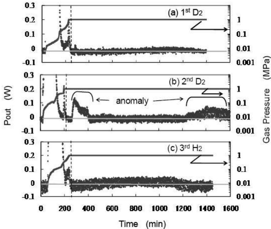
**Figure 11.** Heat power and gas pressure as a function of time for Pd nanopowder AY4030; (a) the first cycle loading with D<sub>2</sub>, (b) the second cycle loading with D<sub>2</sub>, and (c) the third cycle loading with H<sub>2</sub>. The vertical dotted lines indicate the boundary of the first stage and the second stage, and the horizontal gray lines the zero level of  $P_{\text{out}}$ .
