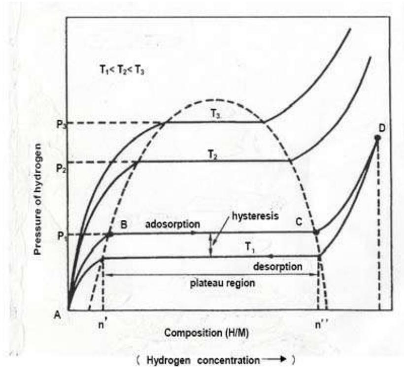
Figure 1. Pressure-composition isotherm adsorption with the parameter, temperature [4].
