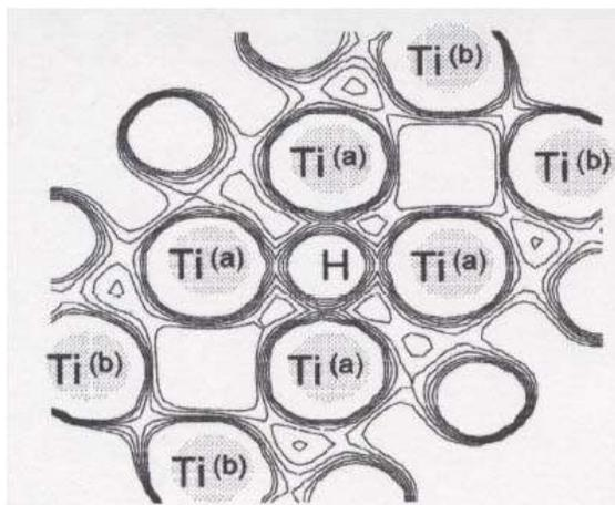
**Figure 8.** The distribution of charge density for (2–203) plane of Ti H<sub>3</sub> (7.69 at.% H) cluster [11].
