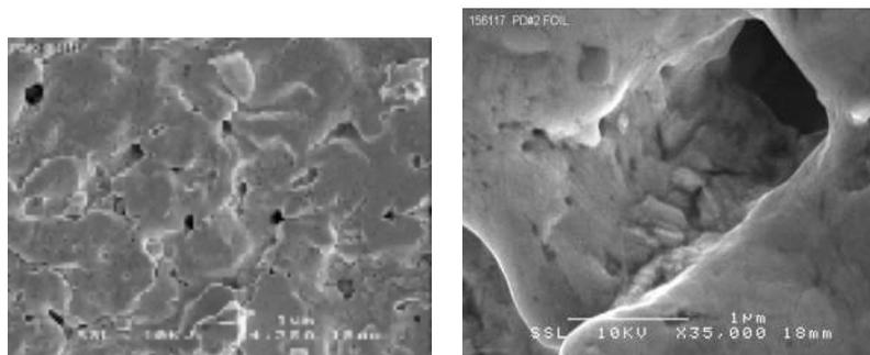
**Figure 4.** a) SEM photo of a Pd target foil ejecta sites at a frequency of 46 kHz shows the ejecta damage to the foil surface. Much milder damage than 20 kHz. SEM photos, Scale  $1\ \text{cm} = 4\ \mu\text{m}$  (b) Detail from 4(a) SEM photo of several square  $\mu\text{m}$  of 4(a) Pd target foil exposed to 46 kHz cavitation shows the diversity of the ejecta population. Scale  $1\ \text{cm} = 1\ \mu\text{m}$ . SEM photos, Jane Wheeler, Evans Lab., Sunnyvale CA. Foil from SRI, Menlo Pk. CA.
