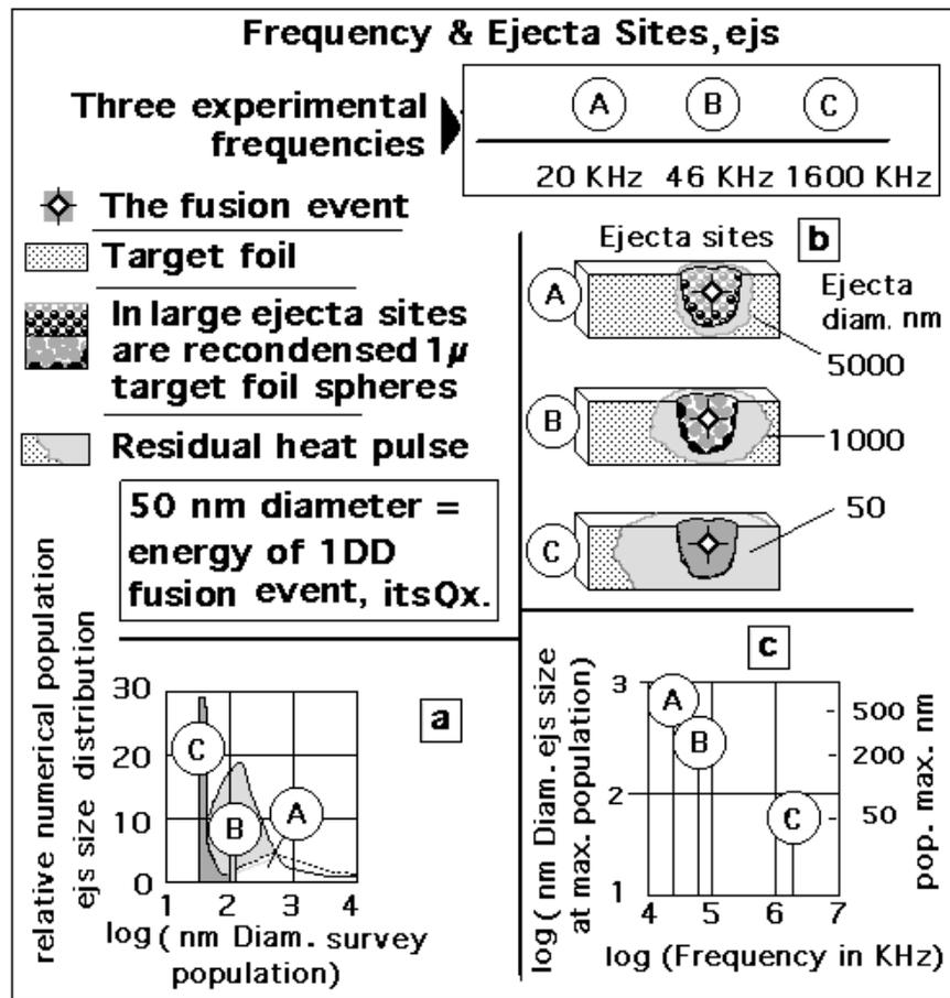
**Figure 2.** a, b, and c. The frequency influences the sizes of the cavitation bubble, the jet, the cluster, the heat pulse, and the ejecta sites. 2a is the ejecta site population distribution. 2b is the ejecta size. And 2c is the population distribution maximum. Ejecta volume is proportional to the cluster fusion events, single or multiple events.
