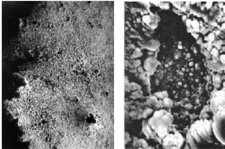
**Figure 3.** a SEM photo of a Pd target foil ejecta site at a frequency of 20 kHz shows the ejecta damage to the foil surface. (Maybe some high density gravitational effects) scale,  $20\ \mu\text{m}$  across. SEM photos 3(a) and (b), John Dash. (b) SEM photo of a detail of 3(a), a large ejecta site, in a Pd target foil exposed to 20 kHz cavitation shows one of the large multi-fusion events showing the  $1\ \mu\text{m}$  diameter sphere debris in the vent. Woodside, CA Lab. 1993.
