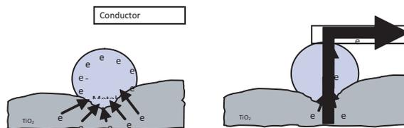
**Figure 2.** Current (electron flow) to a conductor.
