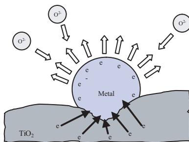
**Figure 1.** Cathodic protection.
