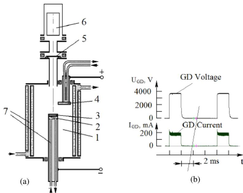
**Figure 1.** Schematic representation of the experiment. (a) Glow discharge device, 1– discharge chamber, 2– cathode holder, 3– cathode sample, 4– anode, 5– Be foil screens, 6– X-ray detectors different kind (pinhole, TLD detectors, scintillator- photomultiplier, spectrometer), objective, 7 –cooling water; (b) Glow discharge voltage and current oscillograms.
