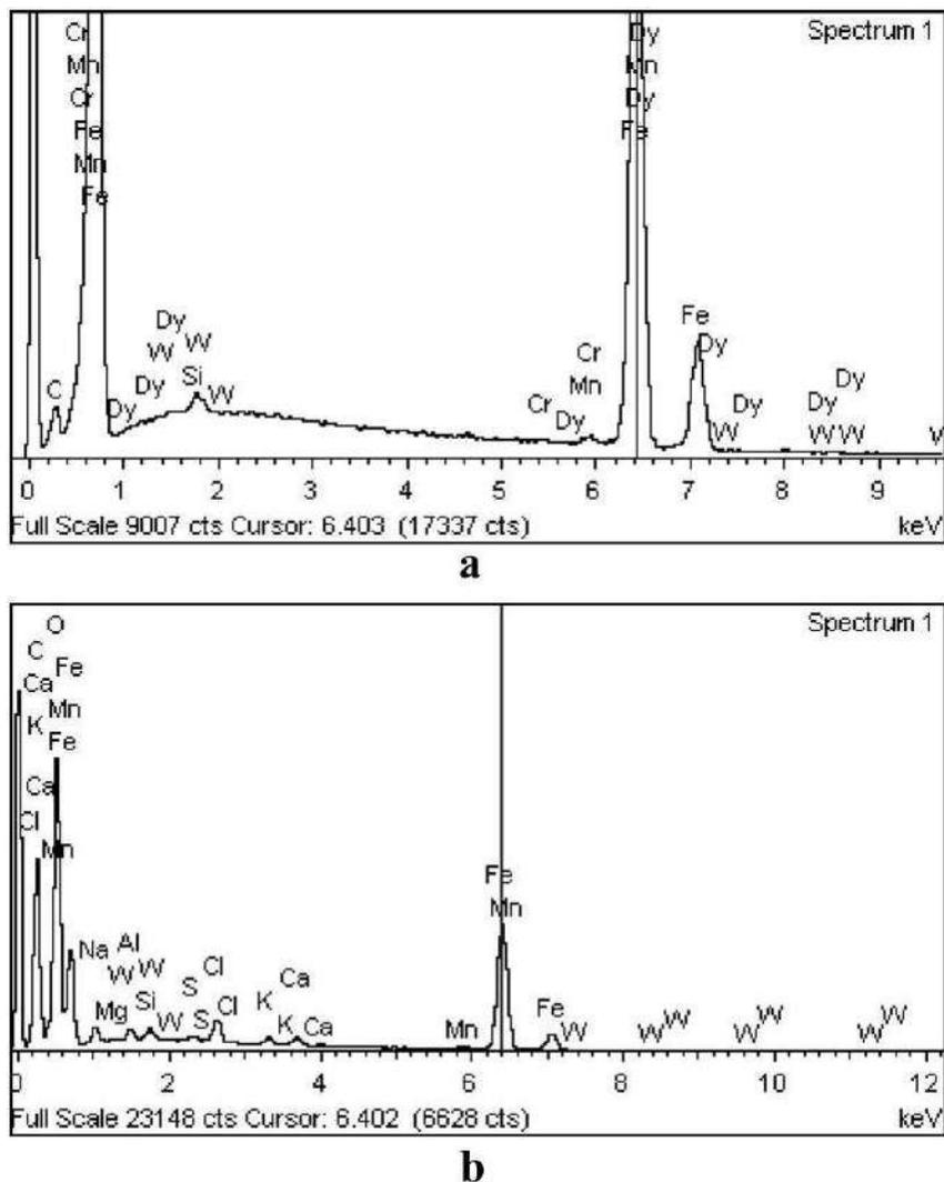
**Figure 5.** Two examples of EDX spectra. In (a) is shown the spectrum of elements on the undamaged part of the surface. In (b) is shown the spectrum of elements on the central spot of one of the circular damaged zones.
