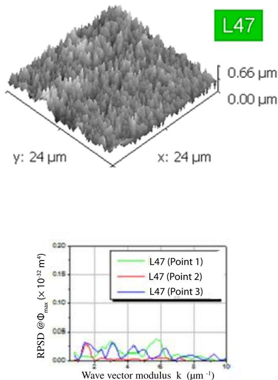
**Figure 3.** Top: 3-D AFM images of samples L47, which did not give excess heat during electrochemical deuterium loading; Bottom: Maximum Power Spectral Density curves computed from the AFM images shown on the top; in case of sample L47 the curves obtained by the analysis of three different sample points are also shown.
