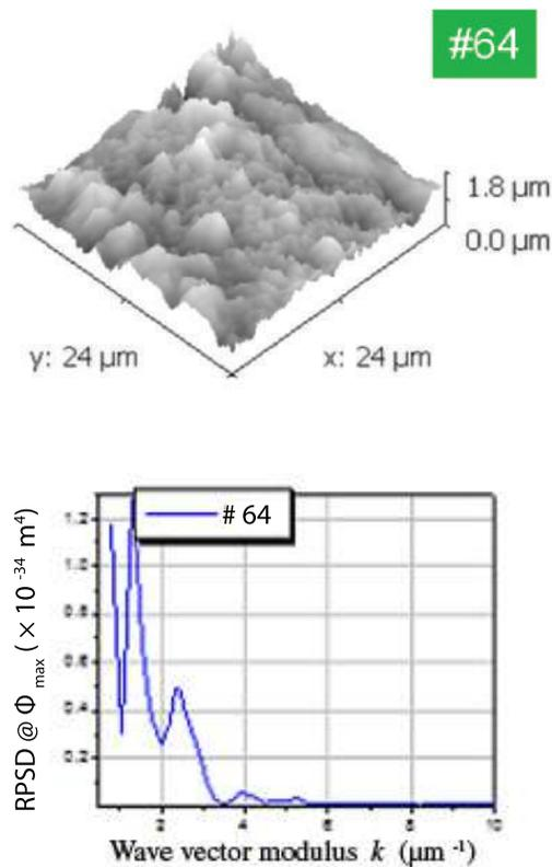
**Figure 2.** Top: 3-D AFM images of samples #64, which gave excess heat during electrochemical deuterium loading; Bottom: Maximum Power Spectral Density curves computed from the AFM images shown on the bottom.
