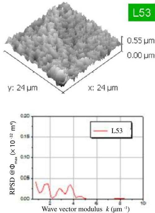
**Figure 4.** Top: 3-D AFM images of samples L53, which did not give excess heat during electrochemical deuterium loading; Bottom: Maximum Power Spectral Density curves computed from the AFM images shown on the top.
