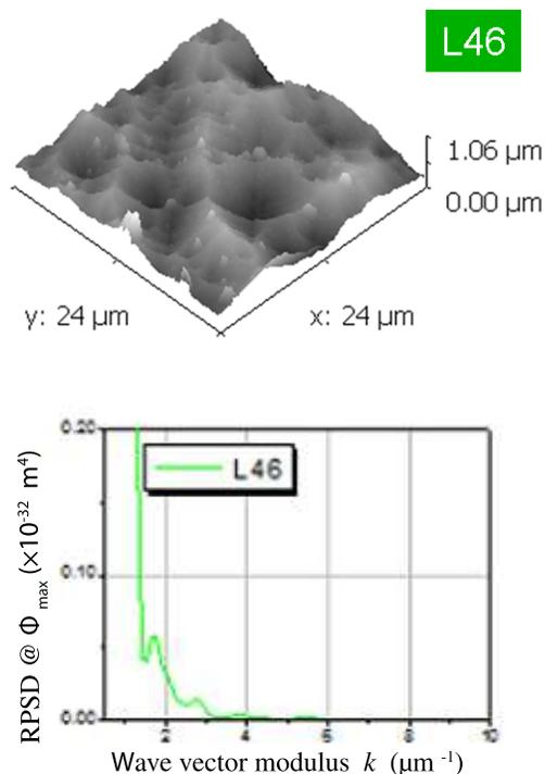
**Figure 1.** Top: 3-D AFM images of samples L46, which gave excess heat during electrochemical deuterium loading; Bottom: Maximum Power Spectral Density curves computed from the AFM images shown on the bottom.
