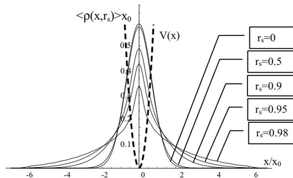
**Figure 5.** Averaged distributions of the probability density  $\langle |\Psi(x, r_s, t \geq 0)|^2 \rangle_t = \langle \rho(x, r_s) \rangle$  for a particle in the same potential well in an area under the barrier for correlated and uncorrelated states of particles with  $r_s = 0; 0.5; 0.9; 0.95; 0.98$
