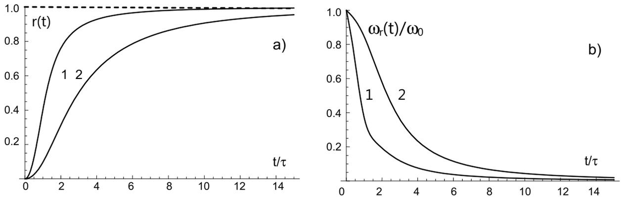
**Figure 1.** Change of correlation coefficient  $r(t)$  of the particle in nonstationary harmonic oscillator (a) connected with the change of frequency  $\omega_r(t)$  of the oscillator (b) for function  $F(t) = c^2 1/c + (\tau/t)^{32/3}$ ,  $c = 2$  (case 1),  $c = 10$  (case 2).
