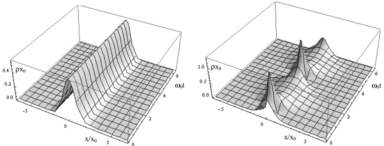
**Figure 3.** Changes of the cross structure of the distribution  $|\Psi(x, r_s, t \geq 0)|^2 = \rho$  in an uncorrelated state  $r_s = 0$ (a) and in a state with the coefficient of correlation  $r_s = 0.9$ (b) in the course of time.
