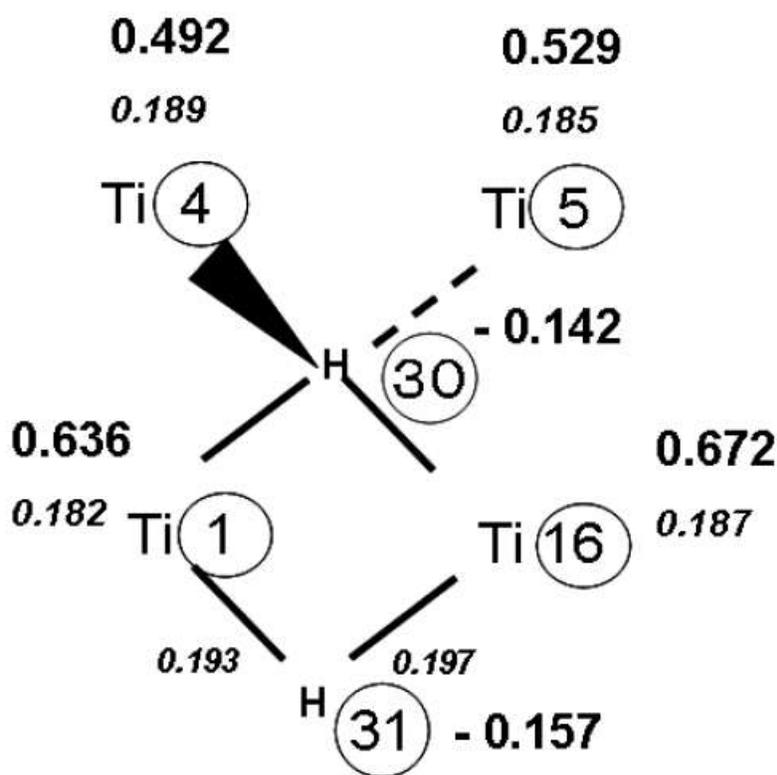
**Figure 4.** Atomic charge value (*bold*) and weighted bond order (*italic*) in the cluster model 3, are indicated in the development drawing of the cluster model 3. Two hydrogen atoms are located inside and outside the cage, respectively.
