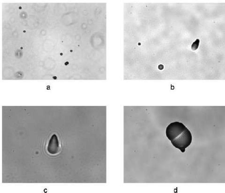
**Figure 5.** Images of tracks in CR-39 detectors created in the course of an experiment: (a) distribution of tracks at 40×, (b) illustrates the angle of impingement at 500×, (c) shows a single track at 1000×, and (d) image of a double track at 500×.
