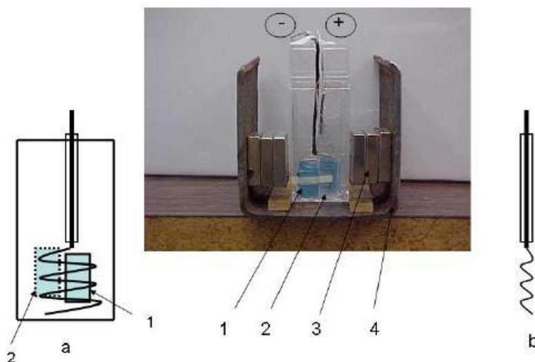
**Figure 4.** Electrochemical cell. (1) Outside CR-39 detector, (2) double CR-39 stock located inside cell, (3) neodymium magnets, (4) magnet holder. Cathode assembly designed for, (a) neutron detection, 1–CR-39 chips inside the cell, 2–CR-39 outside the cell; (b) for determination of deuterium content.
