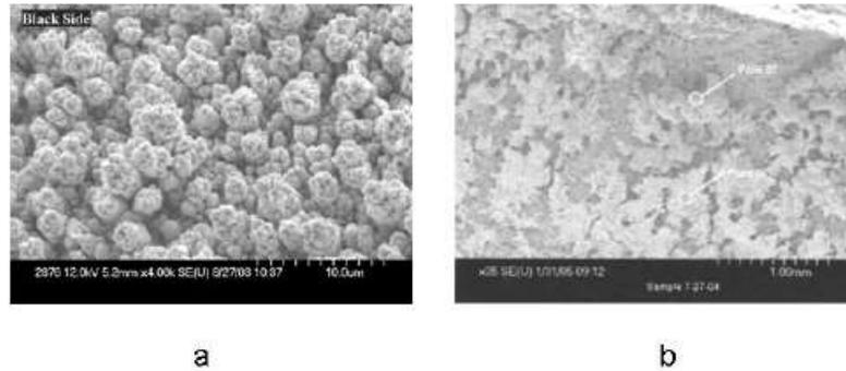
**Figure 1.** (a) SEM photo of electrode surface with no magnetic field applied. (b) Electrode surface with applied magnetic field.
