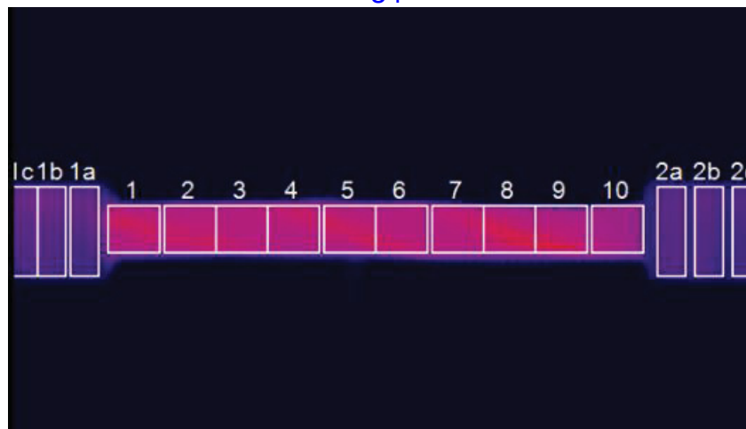
Figure 10. Detail of a thermography image from the dummy reactor run. The image was divided into several areas; the most appropriate emissivity settings were applied to each area.
