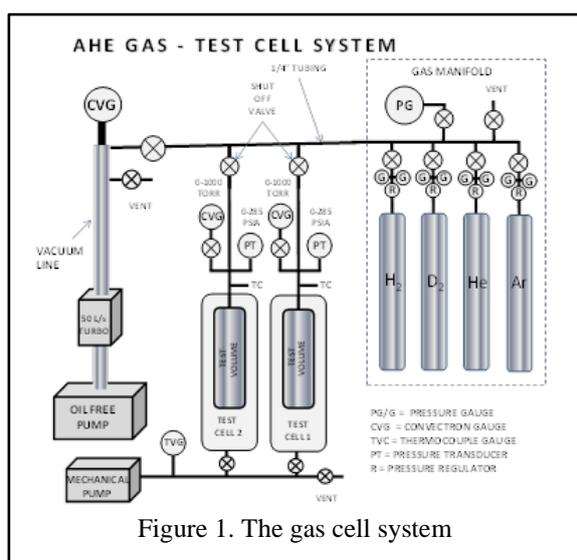
Figure 1. The gas cell system
