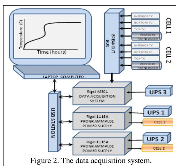
Figure 2. The data acquisition system.
