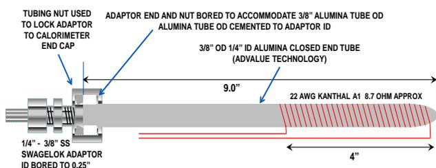
Figure 1. Reactor Design
