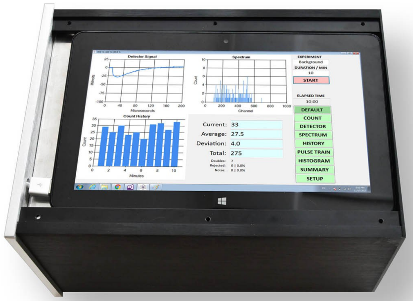
1. Fig. 1. Touch-screen helium-3 neutron detection system with WiFi in Faraday enclosure.
