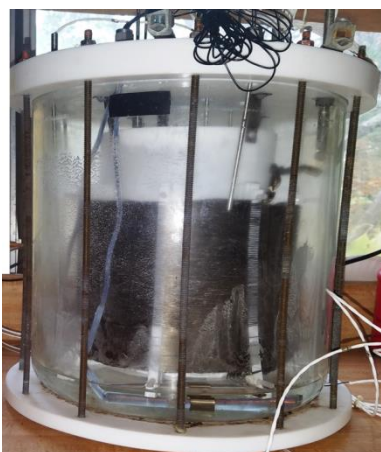
Figure 1 (left) -The electrolytic MOAC ["Mother of all Cathodes"] cell, unfilled; before refilling and adding supplemental diagnostics. Figure 2 (right) - 3/2 [HD/H 2 ] Ratios at various system locations.
