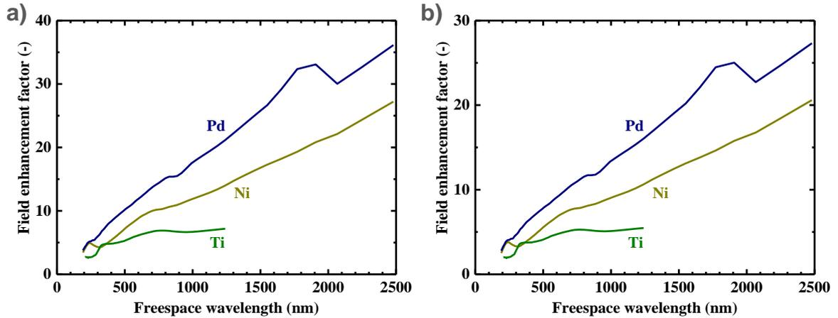
Fig. 1 Field enhancement factors on planar Pd, Ni, and Ti surfaces in (a) D<sub>2</sub>/vacuum and (b) D<sub>2</sub>O.
