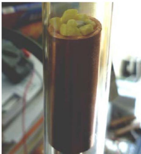
**Figure 1.** Sulfur and lithium atop the anode recess.
