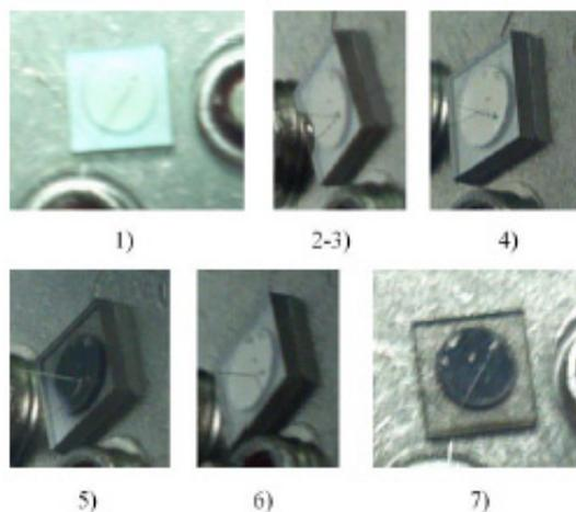
**Figure 3.** Pictures of the electrode on the diamond sensor between each data acquisition from the pressurized hydrogen run. The indexes of the pictures represent the days of exposure that has been completed.
