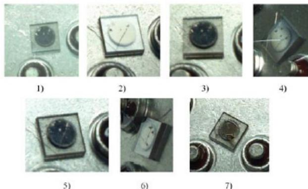
**Figure 6.** Pictures of the electrode on the diamond sensor between each data acquisition from the pressurized hydrogen run. The indexes of the pictures represent the days of exposure that has been completed.
