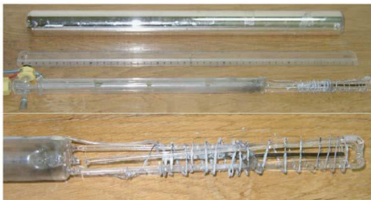
Figure 16. Interior of the cell after the explosion.
