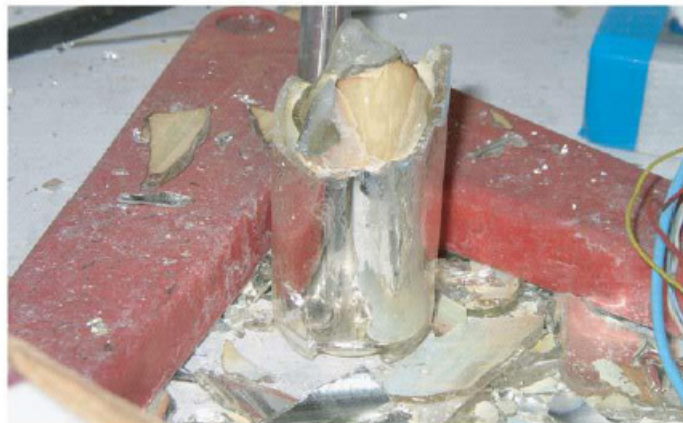
Figure 15. Broken cell after the explosion.
