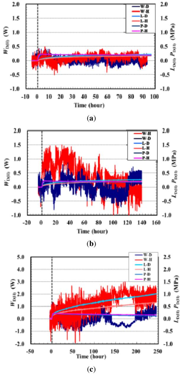
**Figure 6.** Variation of the thermal output power  $W_{D(H)}(t)$ , the pressure  $P_{D(H)}(t)$  and the time-dependent loading ratio  $L_{D(H)}(t)$  in the runs (a) H(D)–NZ3(4)#5\_473 K, (b) H(D)–NZ3(4)#5\_523 K and (c) H(D)–NZ3(4)\_573 K.
