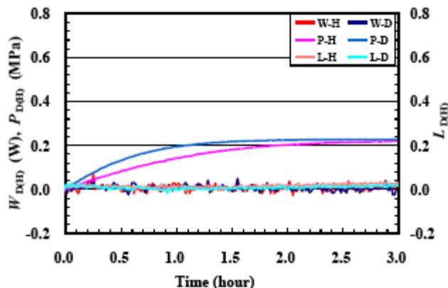
**Figure 7.** Evolution of the thermal power  $W_{D(H)}$ , pressure  $P_{D(H)}$  in the reaction chamber after introduction of  $D_2$  (or  $H_2$ ) gas and the time-dependent loading ratio  $L_{D(H)}$  in runs D–CNZ1#1 and H–CNZ2#1.
