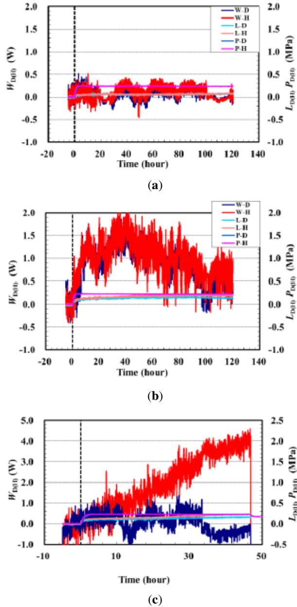
**Figure 8.** Variation of the thermal output power  $W_{D(H)}(t)$ , the pressure  $P_{D(H)}(t)$  and the time-dependent loading ratio  $L_{D(H)}(t)$  in the runs (a) H(D)-CNZ3(4)#5\_473 K, (b) H(D)-CNZ3(4)#5\_523 K, and (c) H(D)-CNZ3(4)#5\_573 K\_2.
