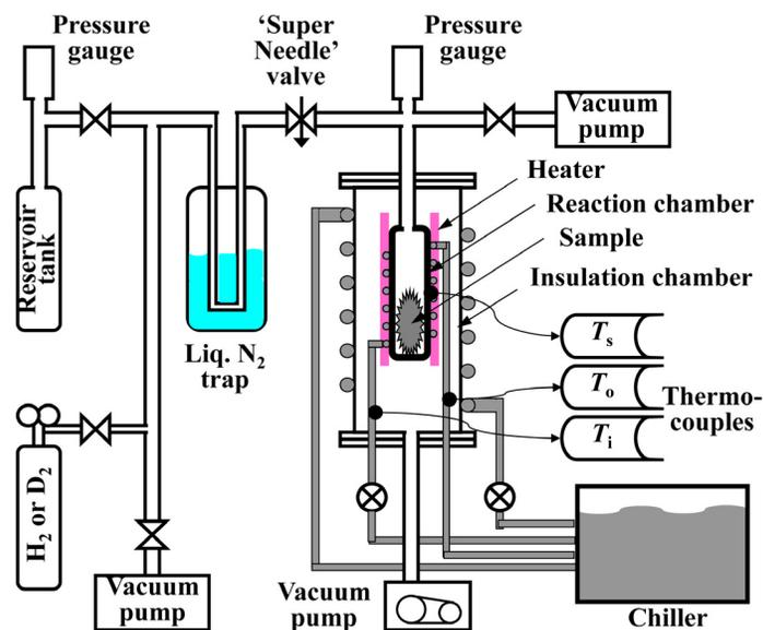
**Figure 1.** Functional view of the system A<sub>1</sub>-A<sub>2</sub>. Water cooling of the reaction chamber with a flow rate of 6 ml/min was done only in the #1 run at room temperature. The cooling water pipe was empty in the #5 runs at elevated temperatures.
