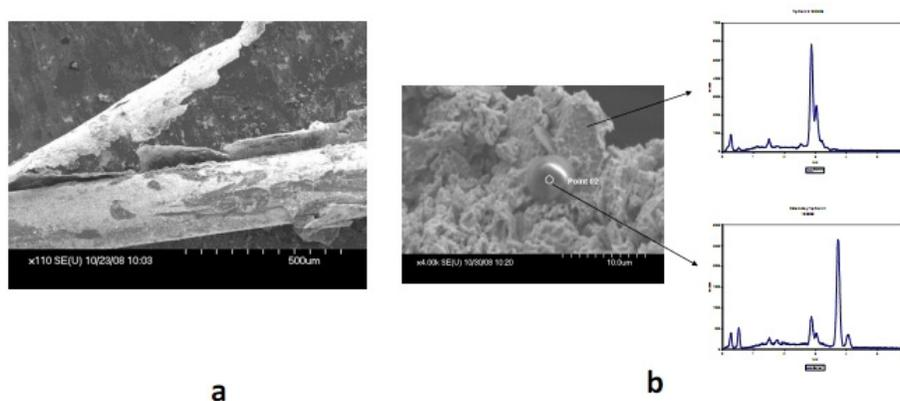
**Figure 10.** SEM/EDX SEM photograph illustrating separation of a Pd/H film during a mild run-a-way run. (a) – SEM photograph showing single reaction site; (c) – EDX of single reaction site (b) showing localized transmutation.
