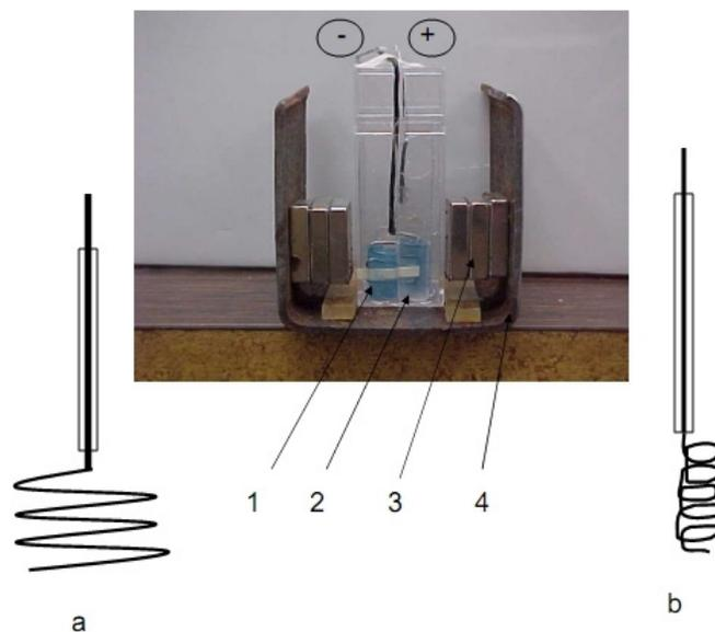
**Figure 4.** Electrochemical cell. 1–outside CR-39 detector, 2 – double CR-39 stock located inside the cell, 3 – neodymium magnets, 4 – magnet holder. Cathode and anode identified by Fig. 1a. Cathode assembly designed for neutron detection, 1 – CR-39 chips inside the cell, 2 – CR-29 outside the cell; Fig. 1b – for determination of deuterium content.
