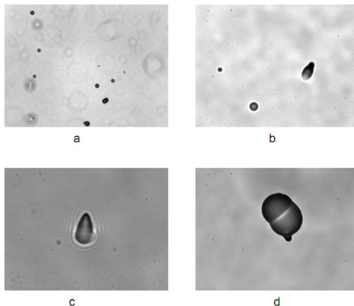
**Figure 7.** Images of tracks in CR-39 detectors created in the course of an experiment; a – distribution of tracks at 40 $\times$ , b – illustrates the angle of impingement at 500 $\times$ , c – shows a single track at 1000 $\times$ , d – image of a double track at 500 $\times$ .
