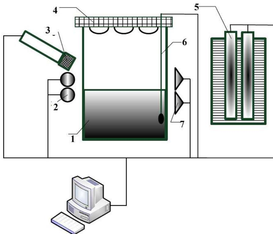
**Figure 1.** Schematic of the experimental configuration. 1–working cell with water solution; 2–Geiger counters type CBM-20; 3–NaI scintillation detector; 4– plate with the sources of red light; 5– $\text{He}^3$  gas neutron counters ( $\text{Ø}3.5 \times 35 \text{ cm}^2$ ) placed in paraffin cylinder ( $\text{Ø}22 \times 40 \text{ cm}^2$ ) or in vessel with water; 6–thermocouple; 7–Geiger counters type CHM-18 with thin window.
