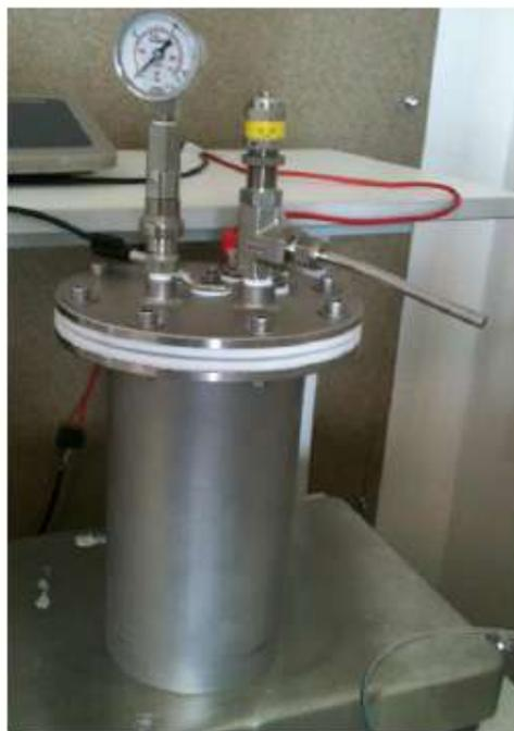
**Figure 2.** A view of the cell on the balance without the insulation blanket.
