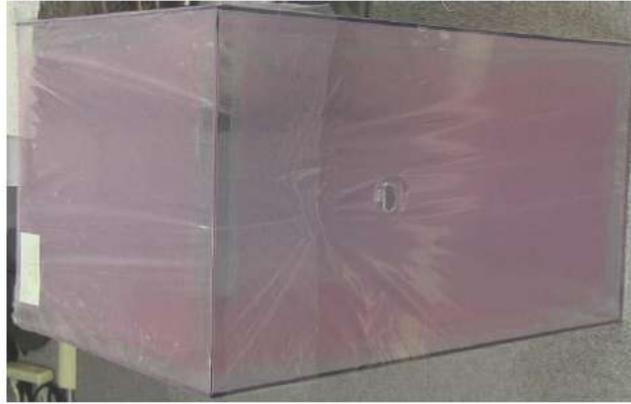
**Figure 12.** Photo of the acrylic calorimeter enclosure.
