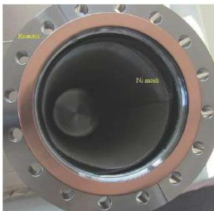
**Figure 3.** View of Ni mesh in the reactor.
