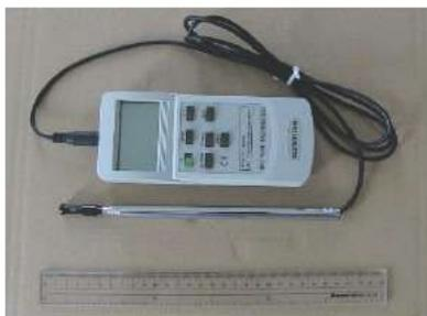
**Figure 15.** Air volume measurement tool for calibration.
