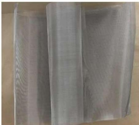
**Figure 2.** Nickel mesh as reactant,  $30\text{ cm}^2$ , 200 mesh. This photo shows the two meshes overlapped.
