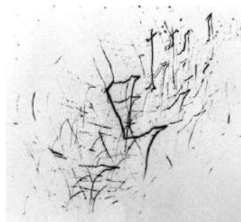
Figure 24. Vector Swarm Group correlation of tracks including random motion components. These tracks do not line up when overlaid. They change form with location, apparently due to relative position in the applied non-uniform magnetic field. A large number of the tracks in this exposure are correlated. A measure of corresponding line segments of matching groups of tracks reveals a macroscopic “central force,” which will be the subject of future work.
