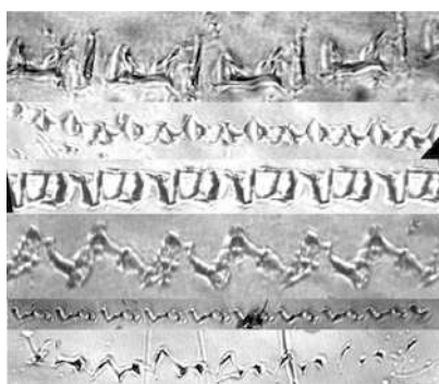
Figure 12. Different types of “evaporated” regular periodic structure tracks in Polychrome Litho film, no pre-exposure, developed with constant agitation.
