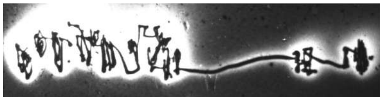
Figure 15. squiggle2 Random motion type tracks in Kodak NTB3 10 \mu nuclear emulsion. Extreme large angle deflections and continuous smooth curvature are shown. Minimum track width = 10 \mu m, track linear measure = 4.3mm.
