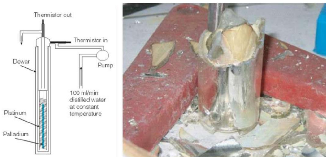
**Figure 3.** Schematic of Biberian's experiment and a photograph after it exploded.
