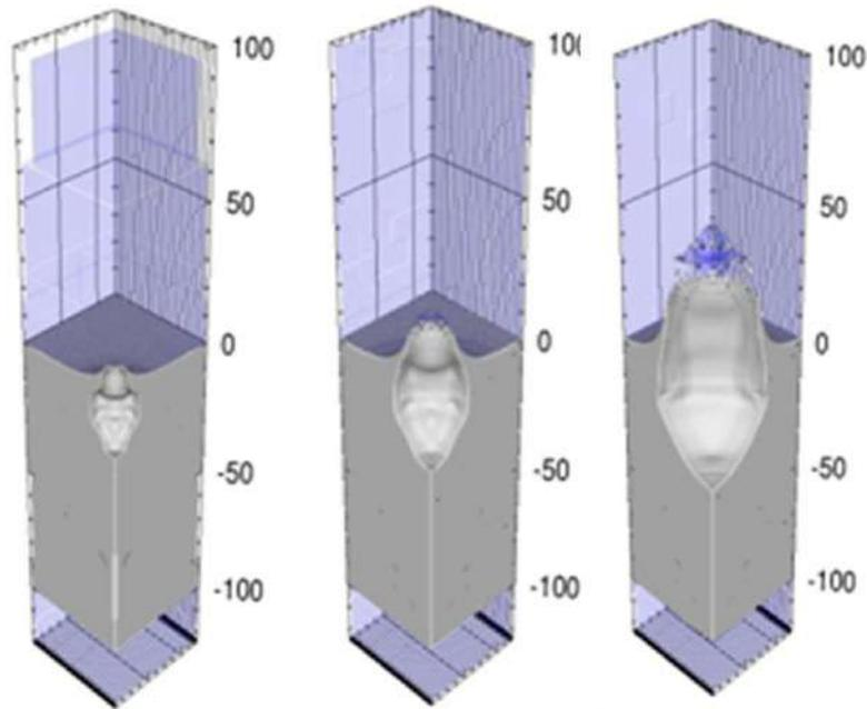
**Figure 5.** Three snapshots at 40, 120 and 360 ns during the evolving dynamics after release of energy in a small volume under the surface of a sample of silver. Only one-fourth of the entire simulation volume is shown for clarity. See text for details and discussion.
