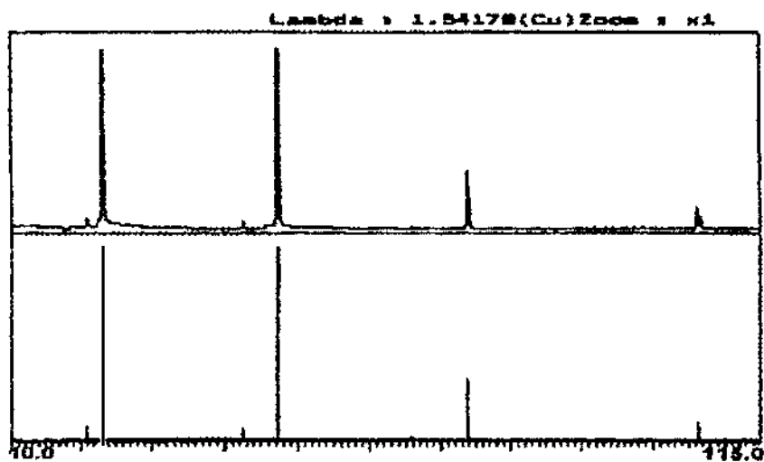
Fig.2. Typical X-ray diffraction pattern for the {100} plane of a cubic sodium tungsten bronze single crystal before experiment. No positive result.
