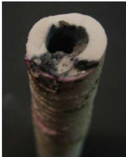
Figure 8. Fragment of the reactor destroyed due to local overheating.
