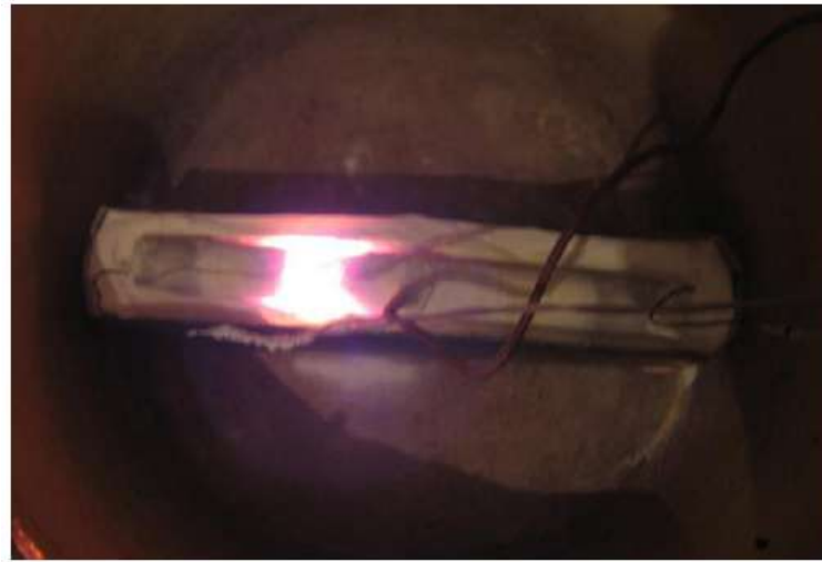
Figure 7. The local overheating that leads to reactor's failure.
